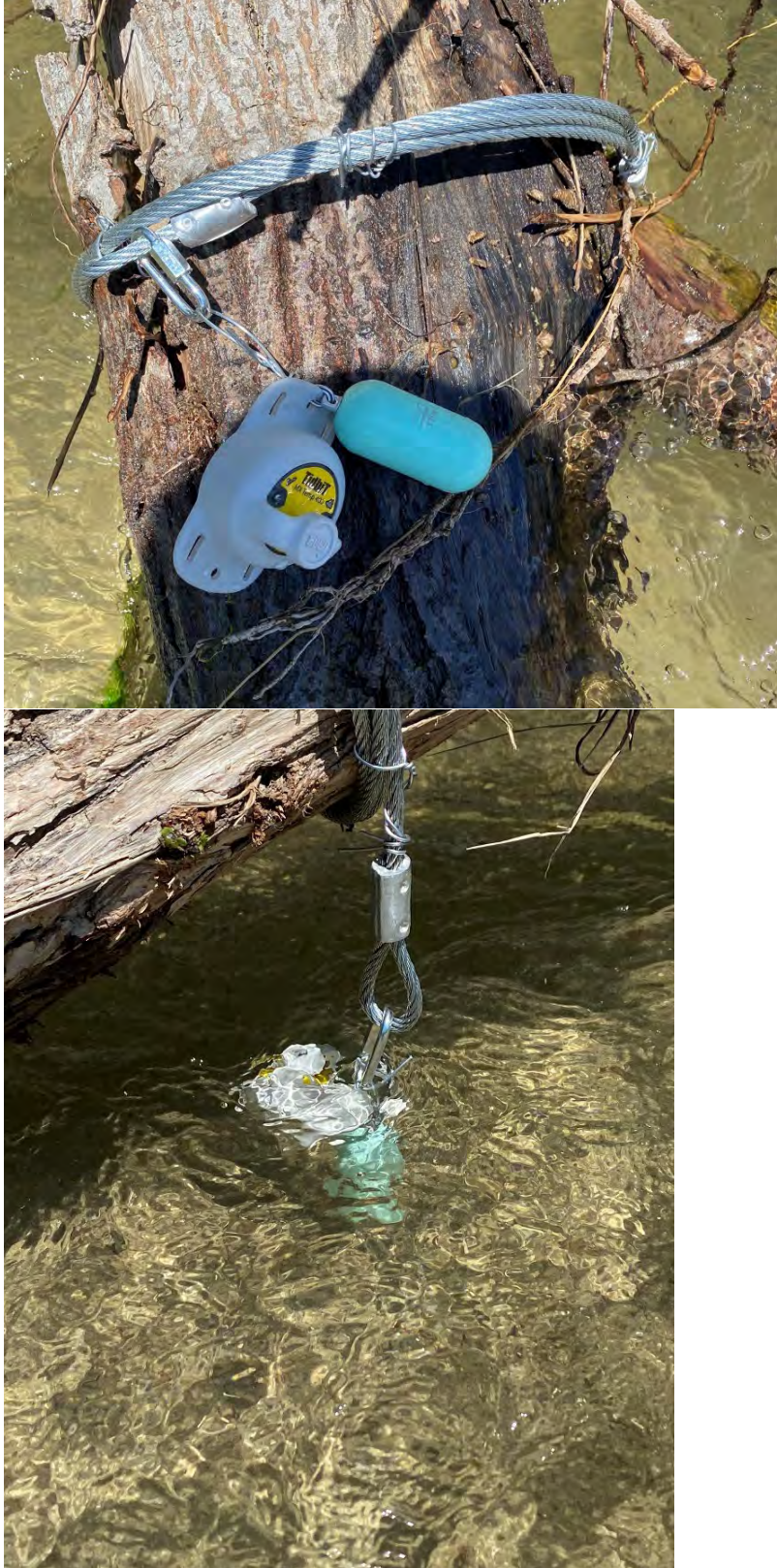
Figure 3-3 Installation of a Temperature Logger on a Submerged Tree Anchor
