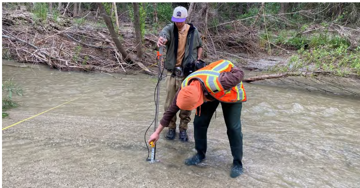
Figure 3-8 Spot Measurements of Velocity and Depth Upstream of the Valencia Water Reclamation Plant
