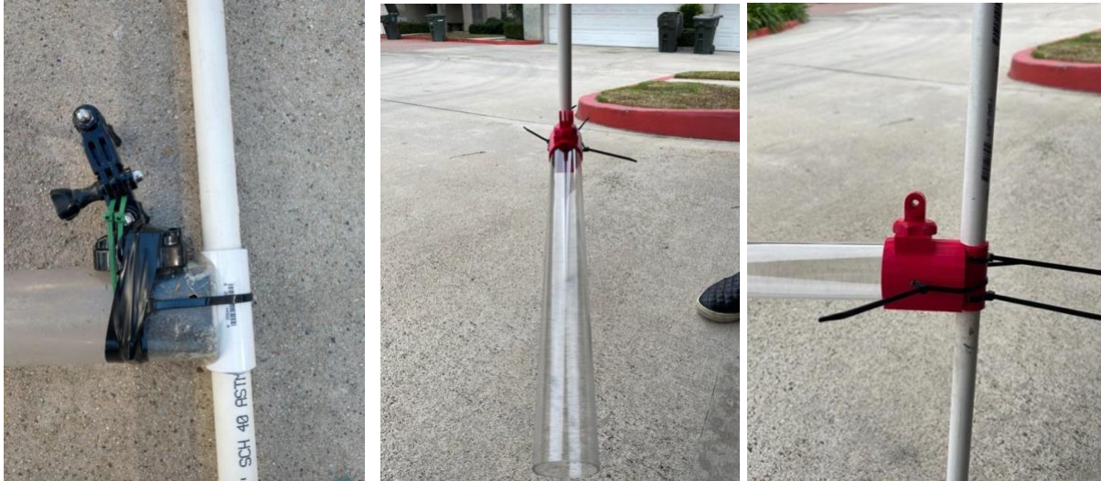
Figure 3. Black tape covering zip ties on BRUV, as well as 3D printed attachment options.
