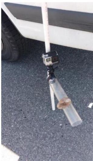
Figure 2. Picture of constructed BRUV with shrimp bait in pantyhose.
