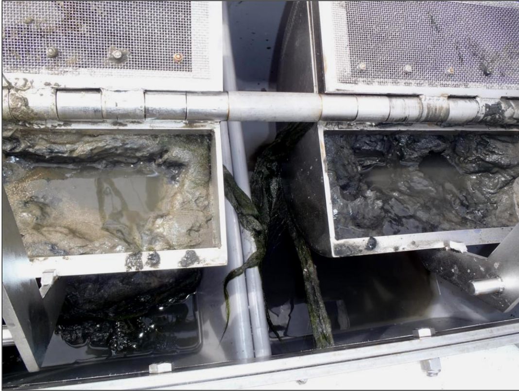
Figure VI-1. Double Van Veen grab sample from Bight'13 sampling showing different sediment types on each side (photo courtesy of AMEC Foster Wheeler).
