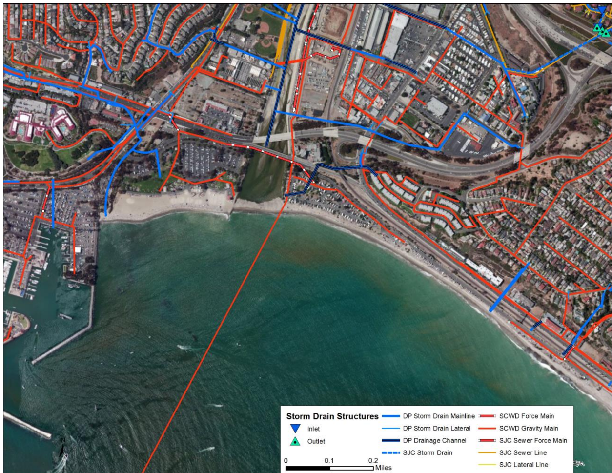
Figure 1. GIS map of Doheny State Beach showing sewer and stormwater infrastructure. DP = Dana Point; SJC = San Juan Capistrano; SCWD = South Coast Water District.
