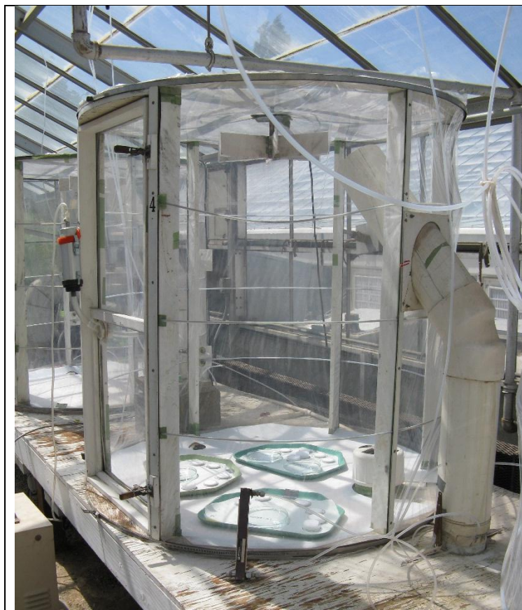
Figure 2.1. Picture of fumigation chamber set up. Three trays were used to evaluate each time point, 24 hours, 48 hours, and 96 hours. A water surface sampler (from which duplicate samples were drawn) and 2 replicate Nylasorb and glass fiber filters were analyzed for each time point. Air concentrations were measured using a denuder system.
