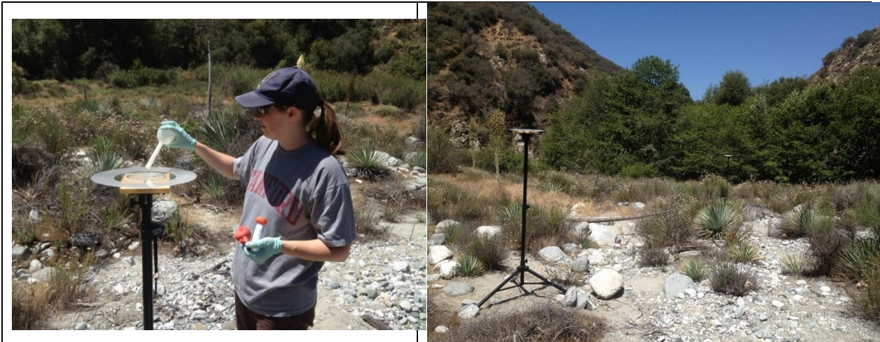
Figure 3.1. Deployment of knife edge surface samplers at Cattle Creek.
