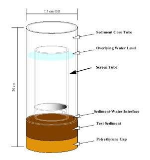
Figure II-2. Schematic diagram of sediment-water interface exposure system (Anderson et al. 1996).
