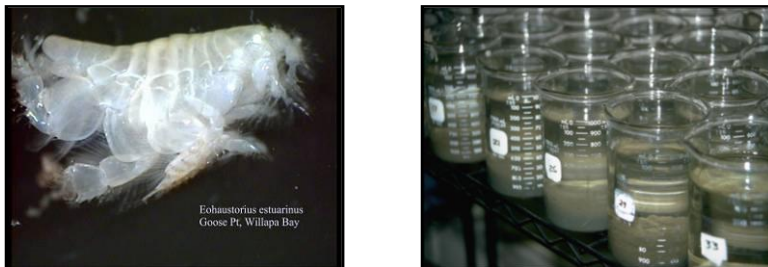
Figure 2. Amphipod ( Eohaustorius estuarius ) used in sediment toxicity tests and exposure chambers.
