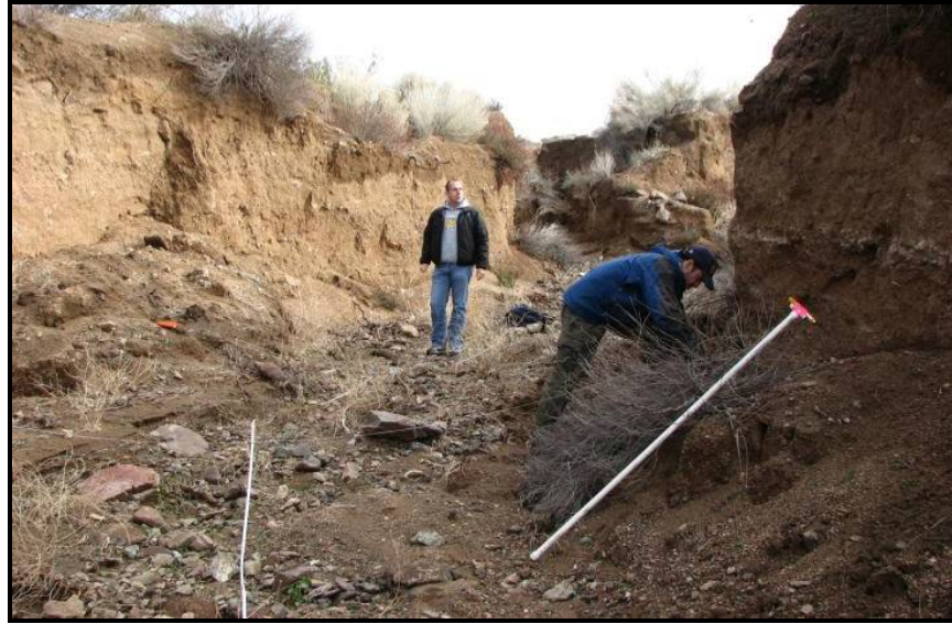
(a) Photograph looking upstream at Acton_D: d_{50} = 9.4 mm with enlargement since development in 1990s approximated at 900%
