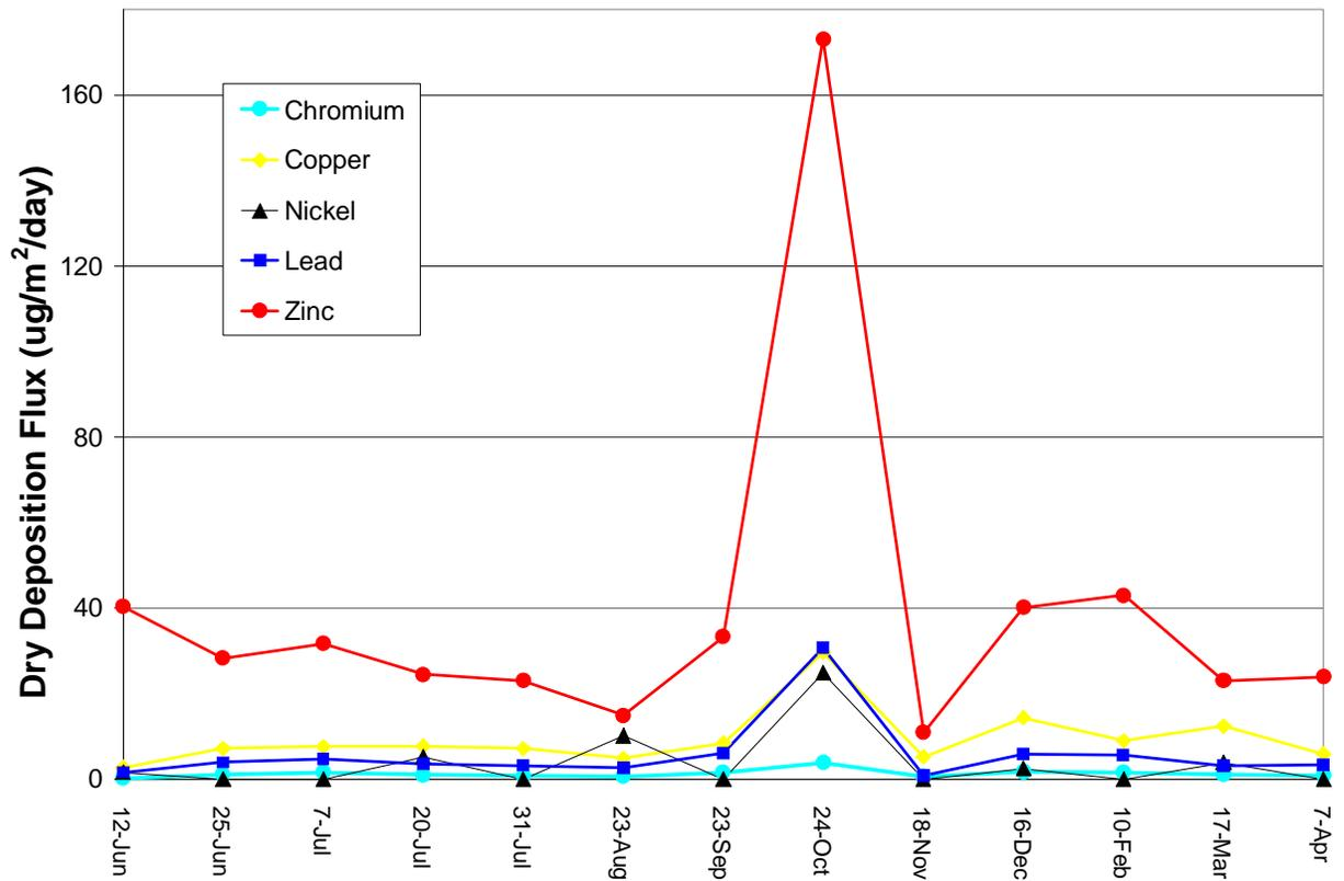
**Figure A-8.** Effect of ash fallout on metals dry deposition flux at the Tillman Wastewater Treatment Plant.
