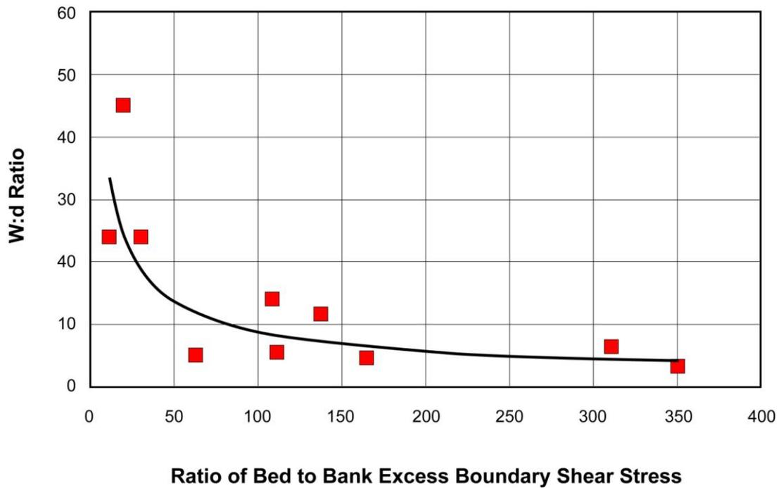
Figure 6-3. Channel Shape and Resistance
