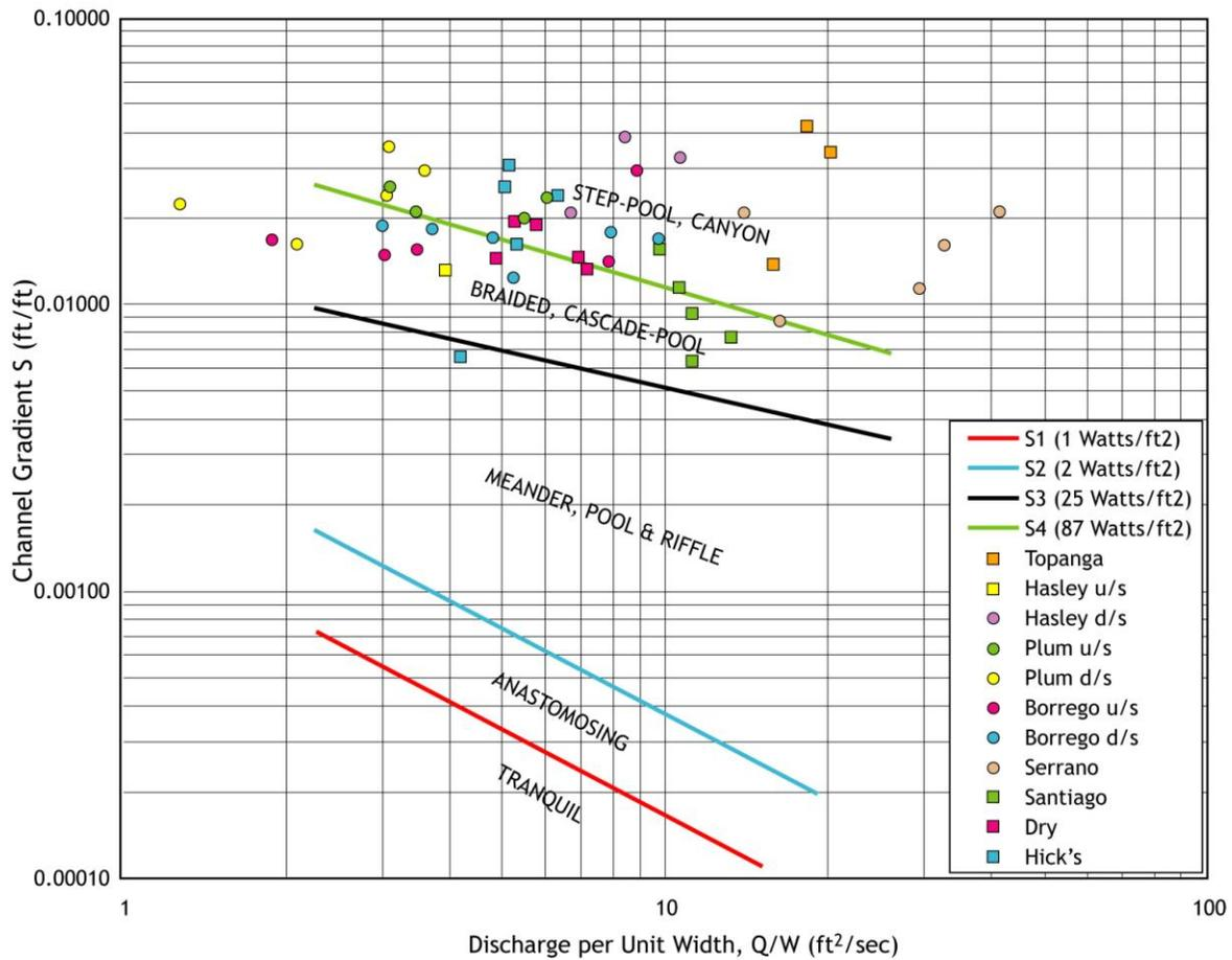
**Figure 4-1. Stream Channel Morphology**
