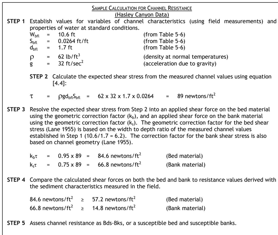
**Figure 4-3. Example Calculation of Channel Resistance**
