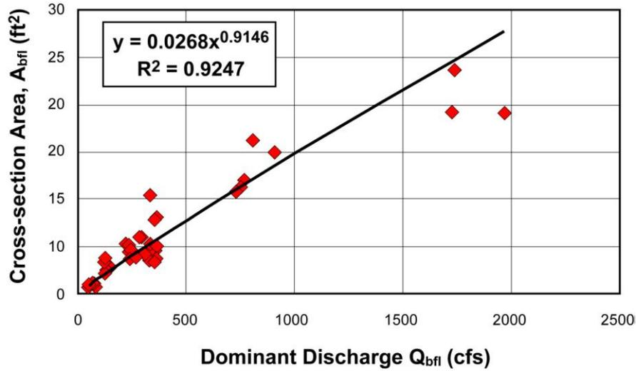
Figure 6-2. Cross Section and Discharge
