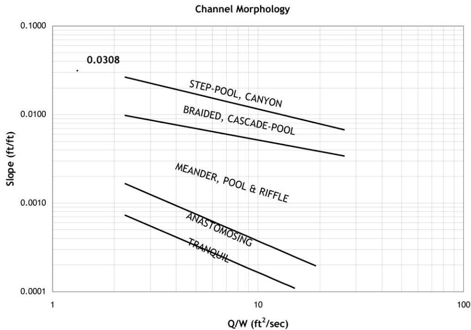
**Step 5** Assess channel form as braided based on plotting position. However, field observations suggest the form is actually a step pool form.
