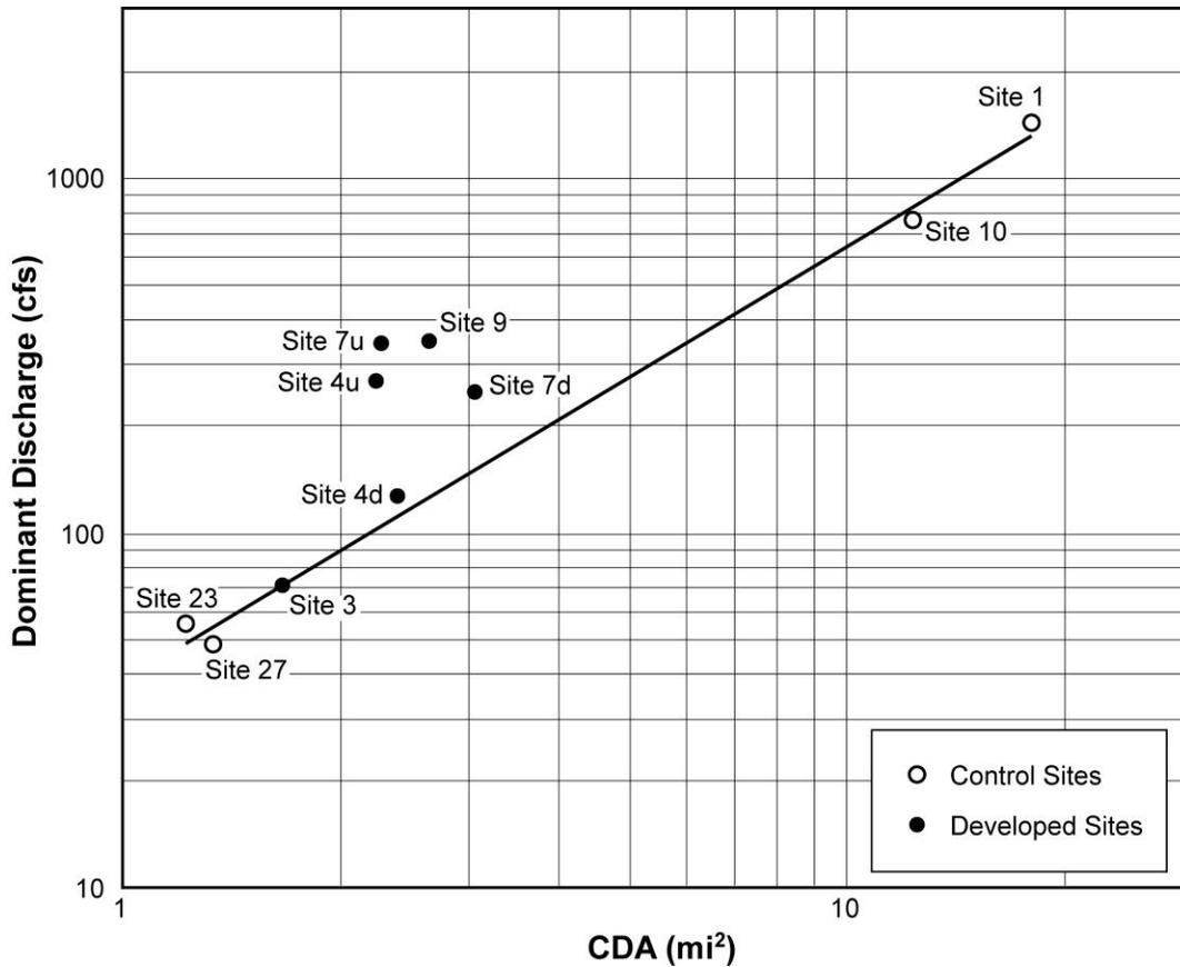
**Figure 5-1. Discharge and Drainage Area**
