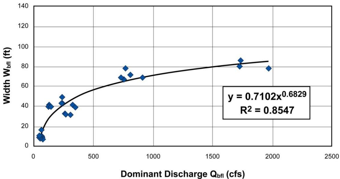
**Figure ES-1: Relationship of Dominant Discharge to Channel Width**
