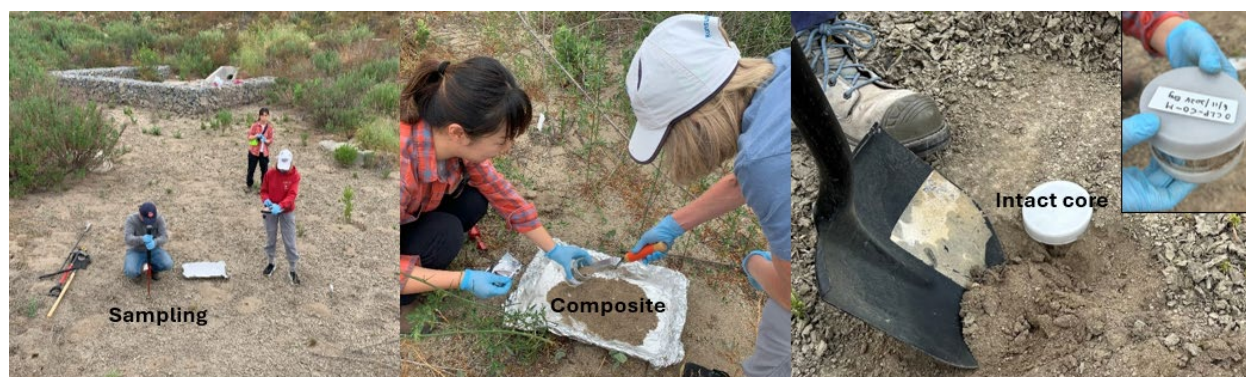
Figure 5. Media collection for composite and intact core samples. Intact cores were used only for measuring media pore-size distribution.
