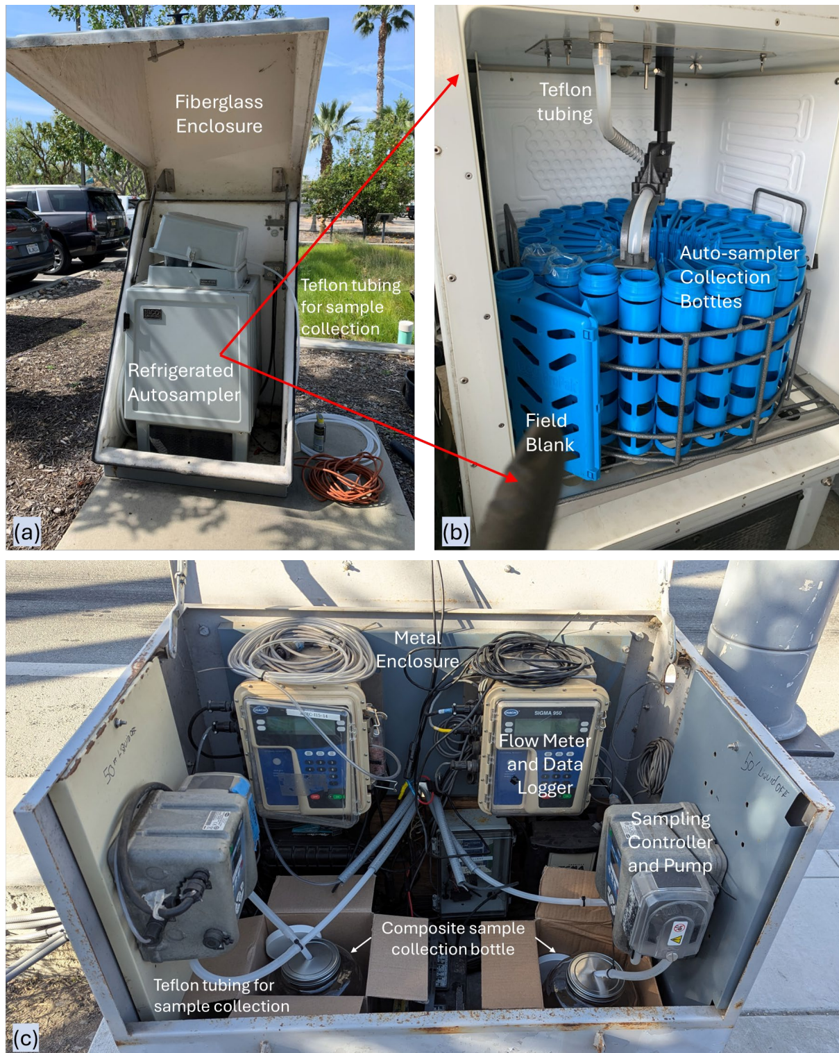
Figure 4. Example instrument configurations used for collecting flow-weighted composite samples of biofilter influent and effluent. (a&b) refrigerated autosampler uses collection “bottles” (in blue) with disposable plastic liners; (c) component equipment for flow and sampling uses a single, large volume, plastic composite sample collection bottle.
