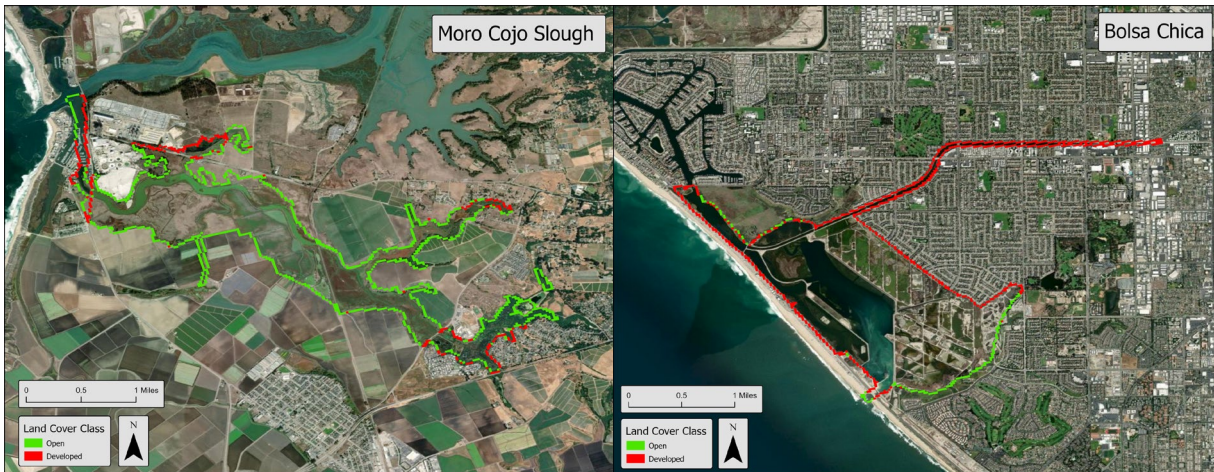
Figure C-9. Example outputs for determining the land use of the immediate wetland perimeter. The NLCD land cover layer was clipped to the 30 m buffer and reclassified into two new groups: open and developed cover.
