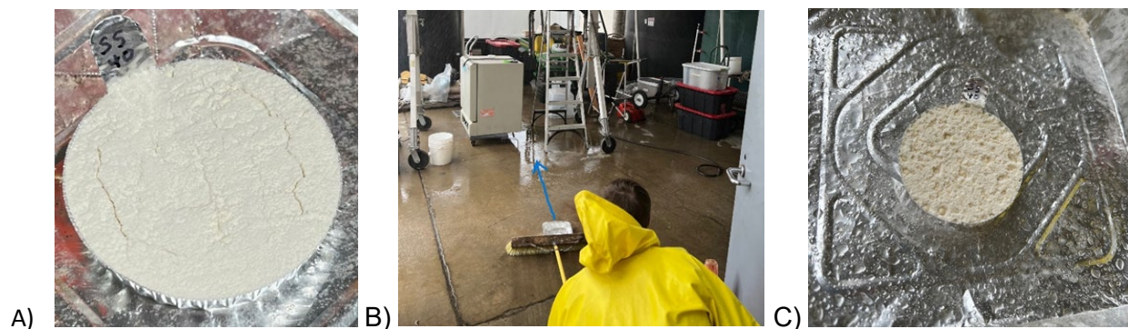
Figure 26. A) Uncompact flour tray; B) Exposing the flour tray to the simulated rainfall for ~1s; C) Droplets’ shape preserved as flour pellets to be dried, sieved, weighed, and counted.
