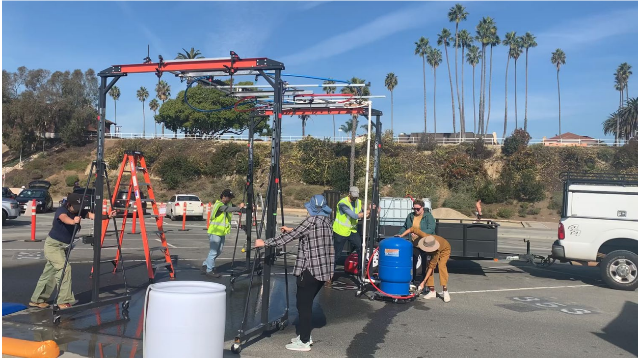
Figure 11. After 15-min of rainfall, the entire RFG and pump assembly are "walked" to the adjacent pavement segment.
