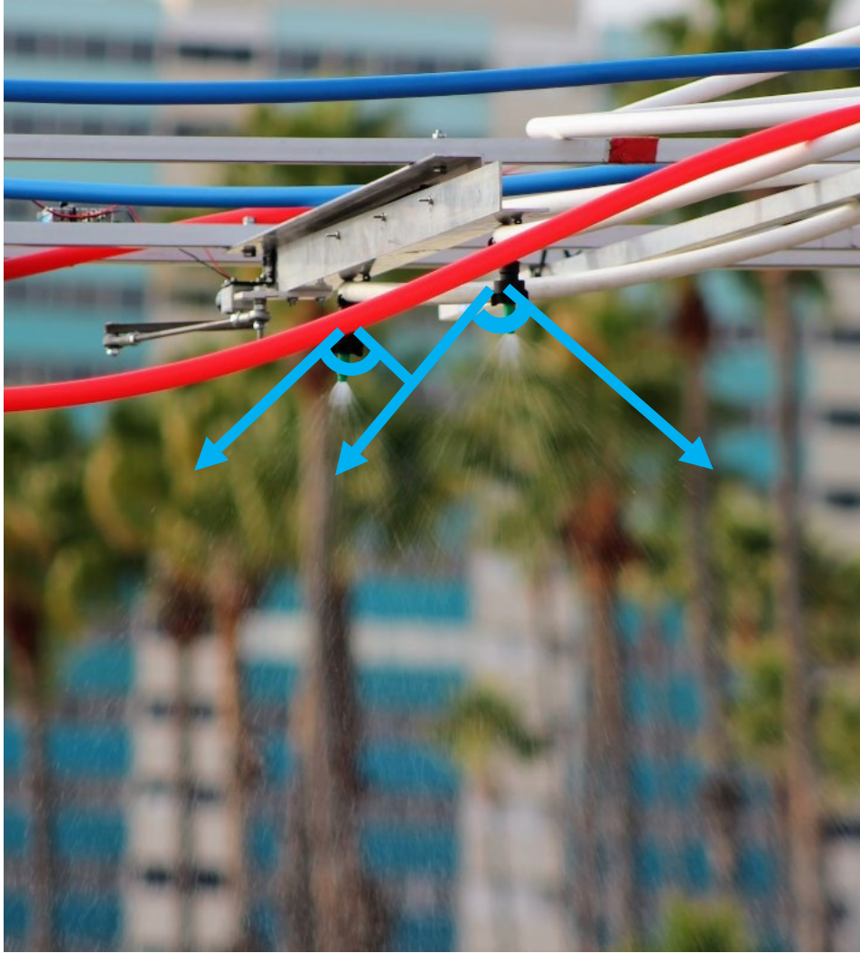
Figure 29. Photograph of AI-TeeJet nozzle spray on the RFG. Spray angle and extents annotated in light blue.
