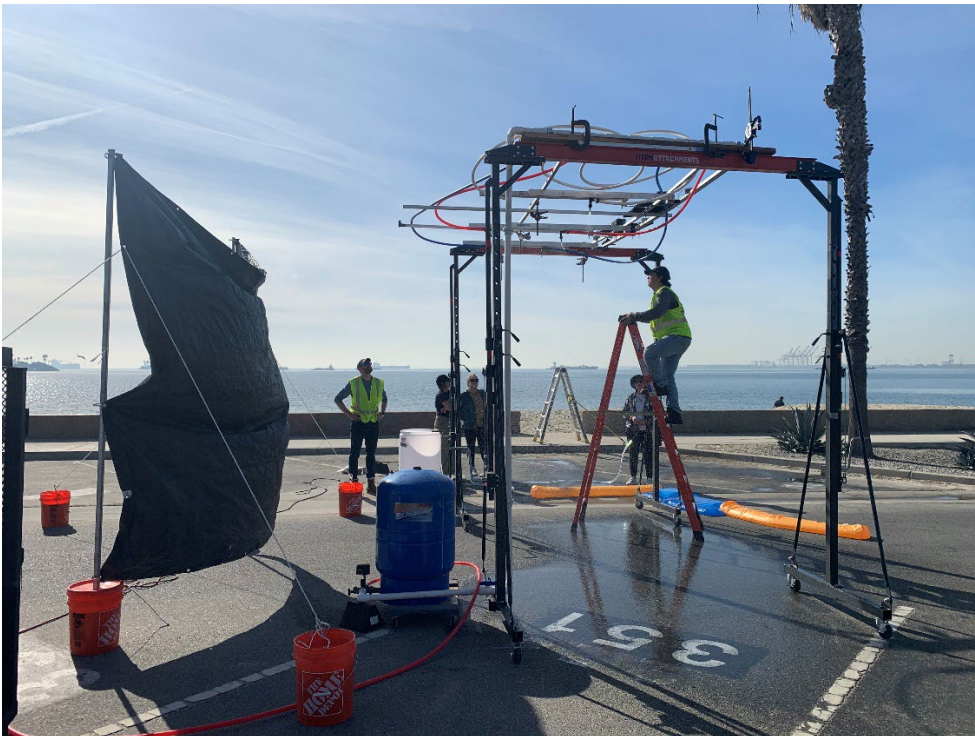
Figure 2. (a) The SCCWRP RFG during shake-down testing showing the full assembly at operational height and with trailer. (b) A windscreen (photo left) was later added to the overall set-up. Ladders are for assembly/disassembly.
