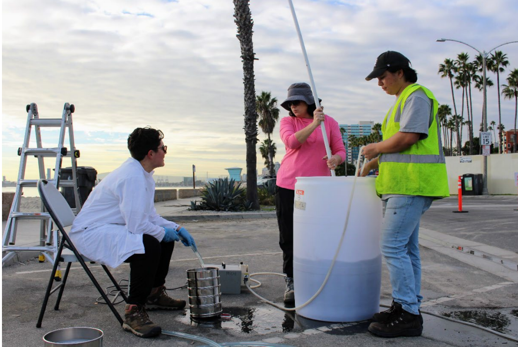
Figure 12. A whole-of-event composite sample is continually mixed while using a peristaltic pump to sieve through a sieve stack to separate particles according to size fraction for microplastics analysis.
