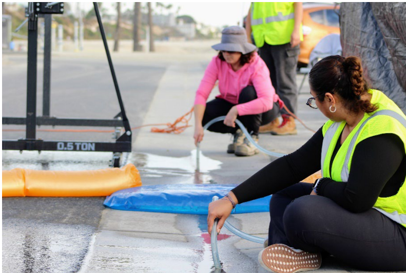
Figure 10. The rainfall generator is positioned close to a gutter pan to facilitate runoff collection. Water-inflatable plastic dams are positioned to promote runoff capture using a multi-channel peristaltic pump. Runoff is collected in a clean 200-L polypropylene barrel.
