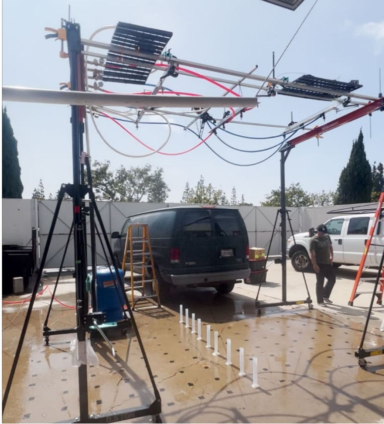
Figure 3. Iterative testing of nozzle position and operating pressure to evaluate simulated rainfall intensity and uniform application (Sept. 2023).
