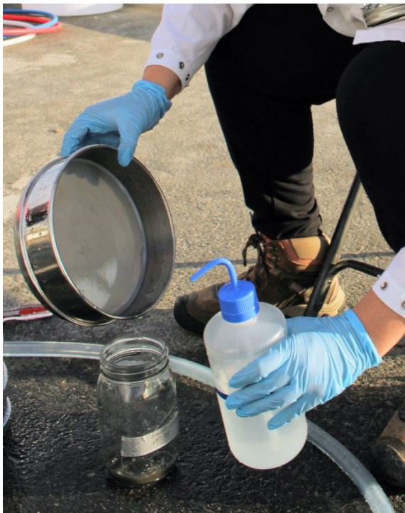
Figure 13. MAG water is used to wash captured particles into a glass jar (1 jar per size fraction) for transportation to SCCWRP and storage until analysis.
