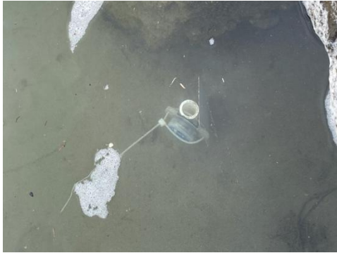
Figure 5.1.7 Hobo tidbit deployed on PVC in shallow estuary.
