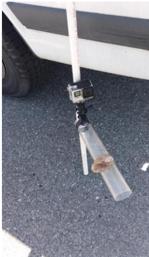
Figure 5.8.2 Picture of constructed BRUV with shrimp bait in pantyhose.
