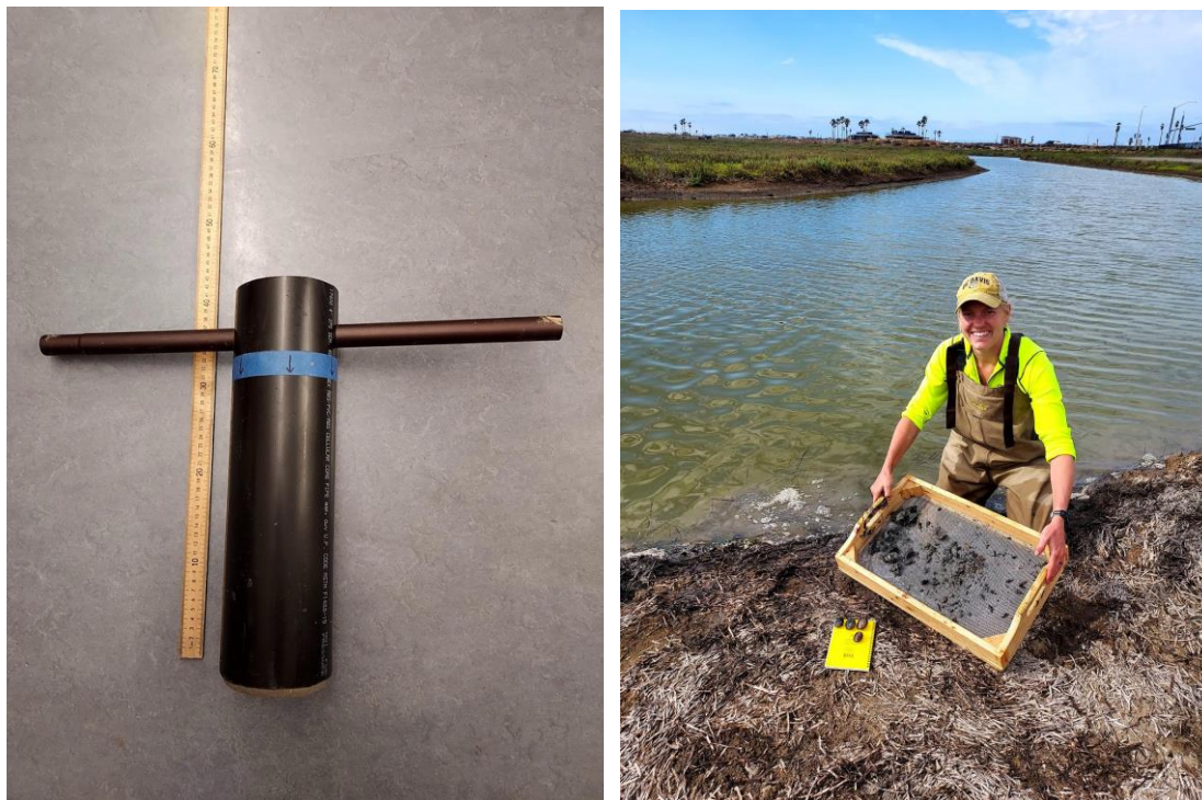
Figure 5.6.3 Example of corer constructed for sampling, and 3 mm sieve being used in Huntington Beach Wetlands to sieve a core.
