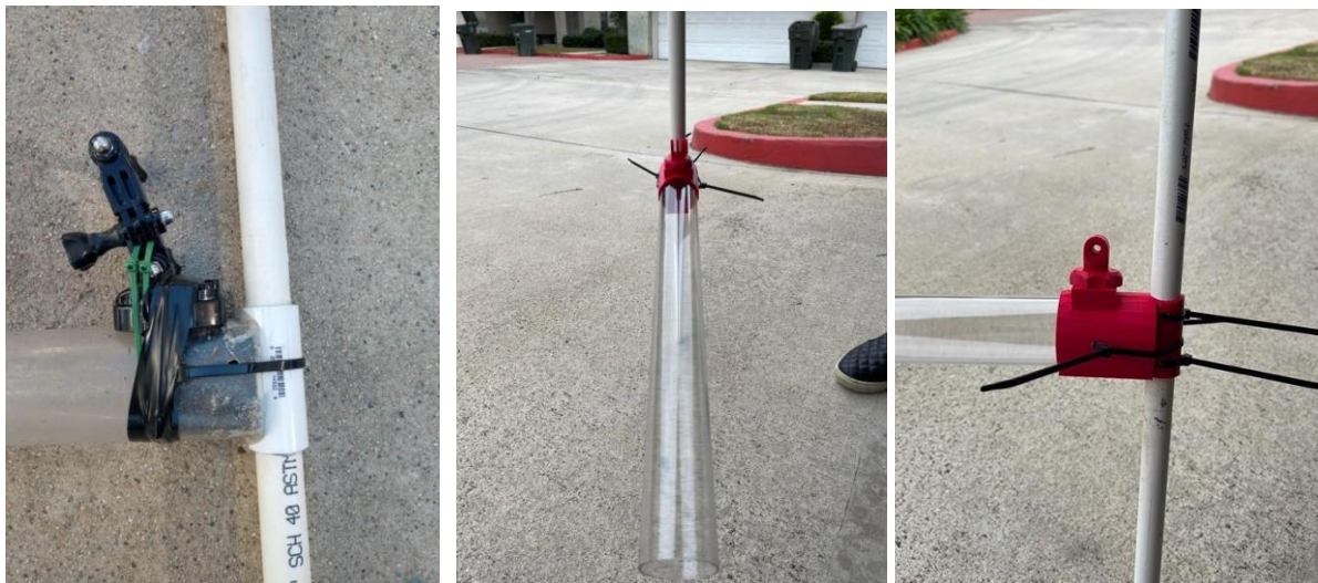
Figure 5.8.3 Black tape covering zip ties on BRUV, as well as 3D printed attachment options.
