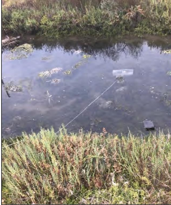
Figure. 5.10.4 In shallow systems, minnow traps can be attached to a single PVC pole and deployed off the channel edge with the PVC anchored into the vegetation [photo: TBF 2021].
