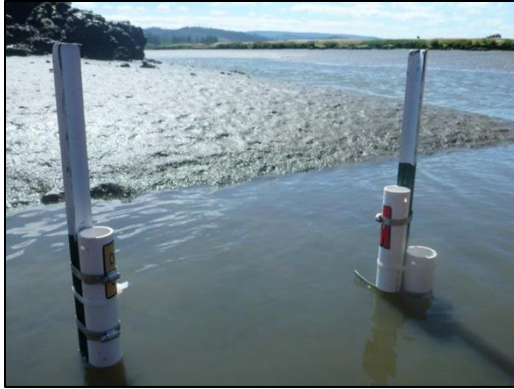
Figure 5.1.6 Example of sensors inside protective PVC tubes (SCCWRP 2015).
