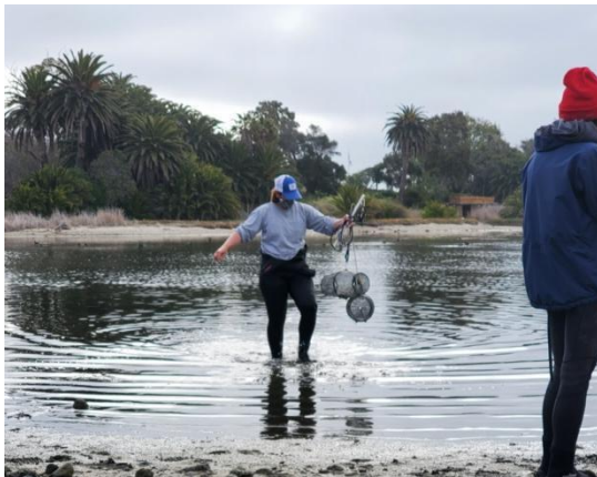
Figure. 5.10.3 In shallow systems, both minnow traps can be attached to a single PVC pole and deployed off the channel edge.
