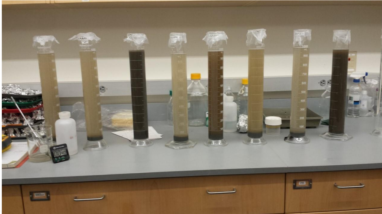
Figure 5.5.1 Graduated cylinders with a range of sediment samples in processing for grain size using hydrometer method. Clear samples are sandier while darker samples have more silt and clay. Photo: C. Whitcraft
