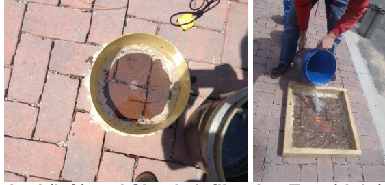
Figure 9. ASTM C1701 standard (left) and Simple Infiltration Test (right) SIR measurement methodologies.
