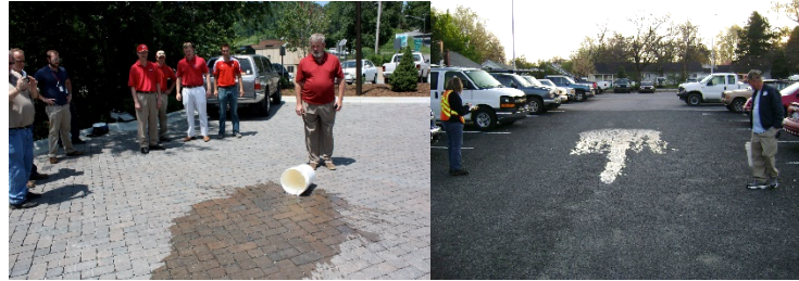
Figure 8. Examples of a successful (left; note infiltration at point of water application) and a failed bucket test (right; note runoff plume).
