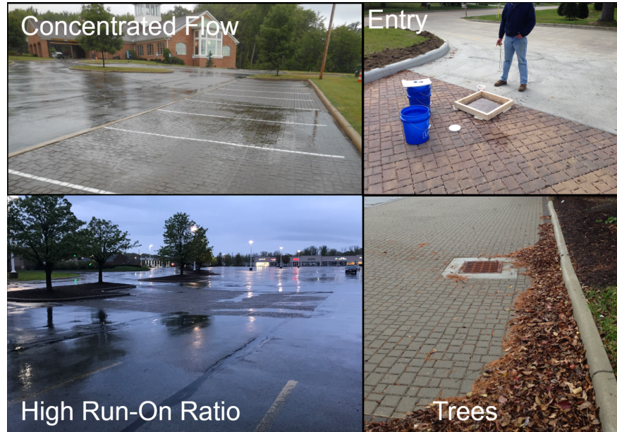
Figure 4. Clogging stimuli tested at permeable pavement sites in Ohio.
