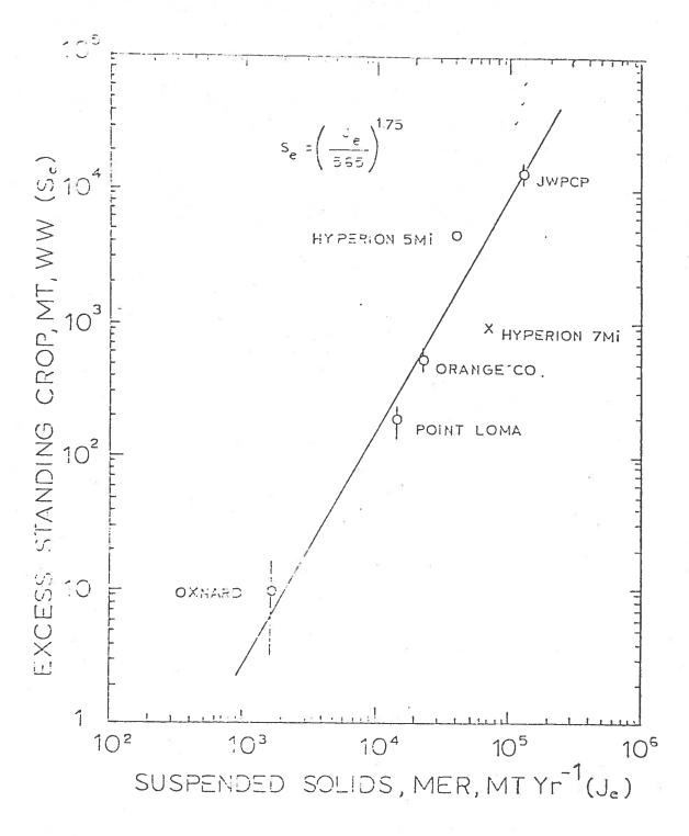
Figure 7. Relationship between suspended solids mass emission rates (Us) and area occupied by excess standing crop (Ae) at six southern California ocean discharge sites. Open circle and bar represents median and range of estimates of area; x represents estimate of size of affected area near the Hyperion 7-mile sludge outfall (excluded from regression line).
