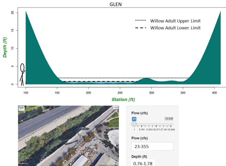
Figure 7. Dry-season flow range for willow adult at GLEN plotted on the channel cross section to visualize corresponding depth and wetted width of the upper and lower limits adapted from the beta R Shiny App ( https://mohammap.shinyapps.io/LAVIS/ ).
