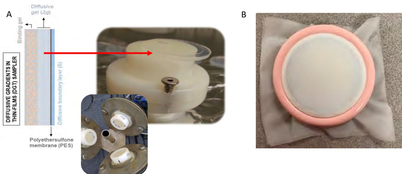
**Figure 2. Schematic of an o-DGT passive sampling device (A) and a SPATT bag (B).**
