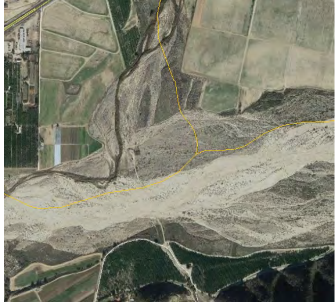
The stream has migrated away from the flow line. In this case, the inaccuracy is not significant, as the flowline characterizes a similar setting to the stream's true location. Constraint classifications won't be affected.
