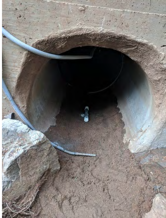
Figure 3. Pictures clockwise from top left; LC8F discharge during dry weather, LC8F discharge flowing; LC8F discharge with sampling tubing and flow meter instrumentation installed.
