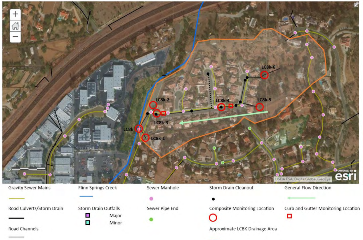
Figure 9. Map of sampling locations for Storm 3 at LC8K. Monitoring locations are described by red circles, sanitary sewer manhole covers are pink dots, flow direction is shown as a green arrow, and the drainage area is outlined in orange.
