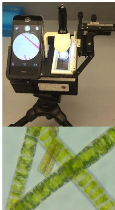
**Figure 3.** The SCCWRP CellScope, developed in collaboration with UC Berkeley, and a sample specimen image captured with an iPhone.
