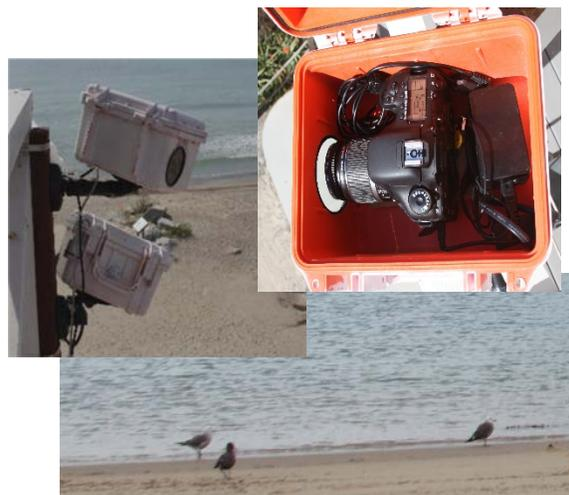
**Figure 4.** A computer controlled, high-frequency DSLR camera system deployed at Doheny State Beach collected images every three minutes to assess bird activity and density on the beach via change detection algorithms developed in MATLAB.
