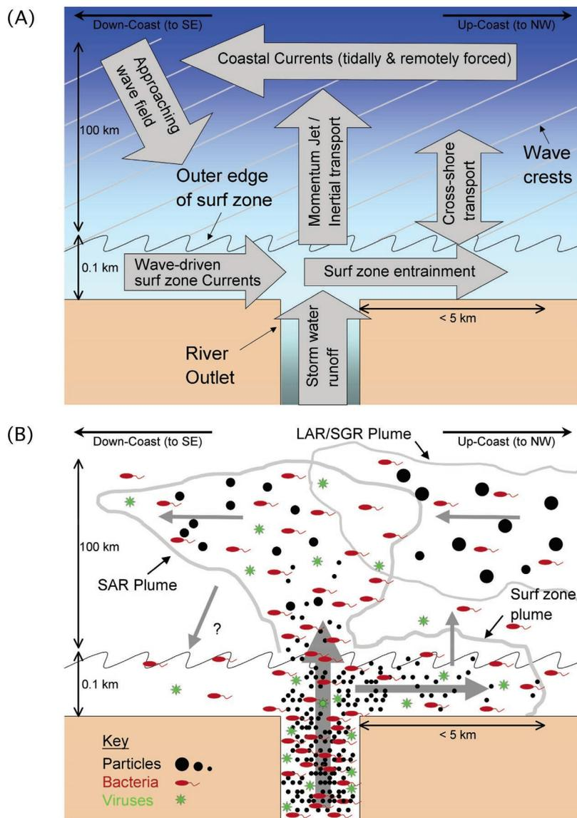
**FIGURE 8. (A) Transport mechanisms that can affect the offshore distribution of contaminants discharged from river outlets. (B) Schematic representation of the spatial distribution of particles (black circles of varying size), fecal indicator bacteria (red symbols), and F<sup>+</sup> coliphage and human pathogenic viruses (green symbols). Abbreviations are SAR (Santa Ana River), SGR (San Gabriel River), and LAR (Los Angeles River).**
