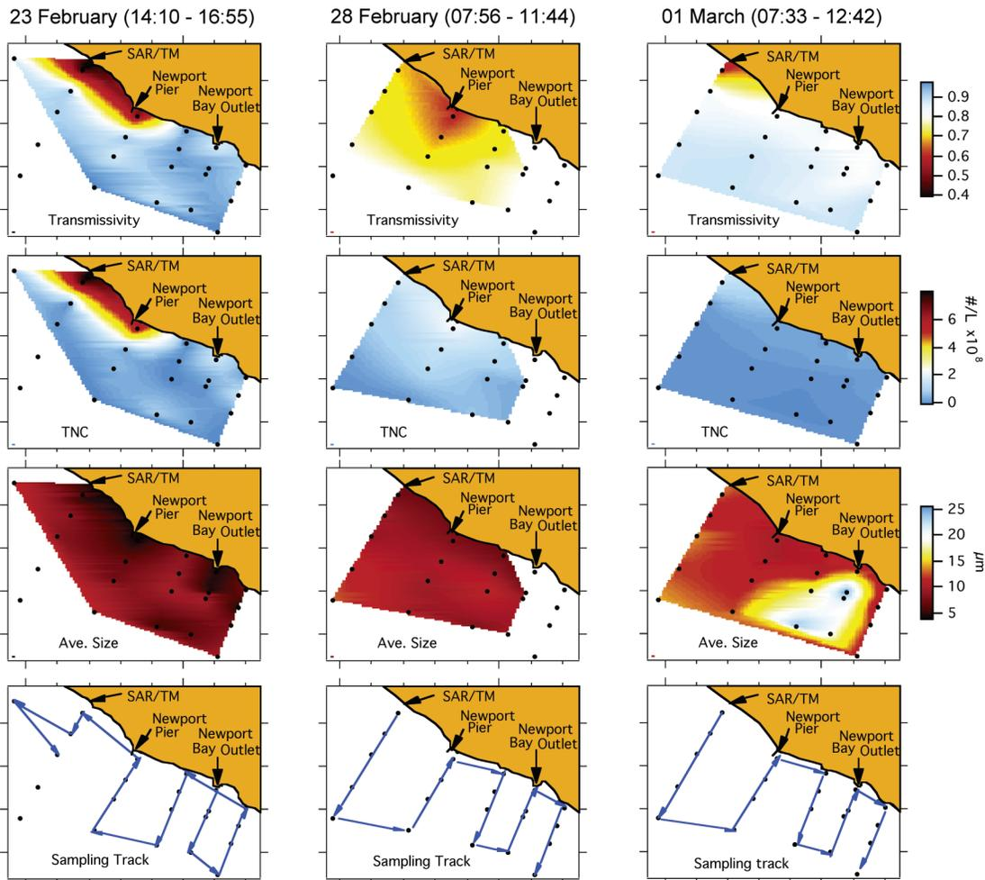
**FIGURE 4. Particle measurements collected during the three sampling cruises. The bottom row of panels indicates the sampling track. TNC is an abbreviation for total particle number concentration. TNC and number-averaged particle size were calculated from measured particle size spectra using eq 1a, b.**
