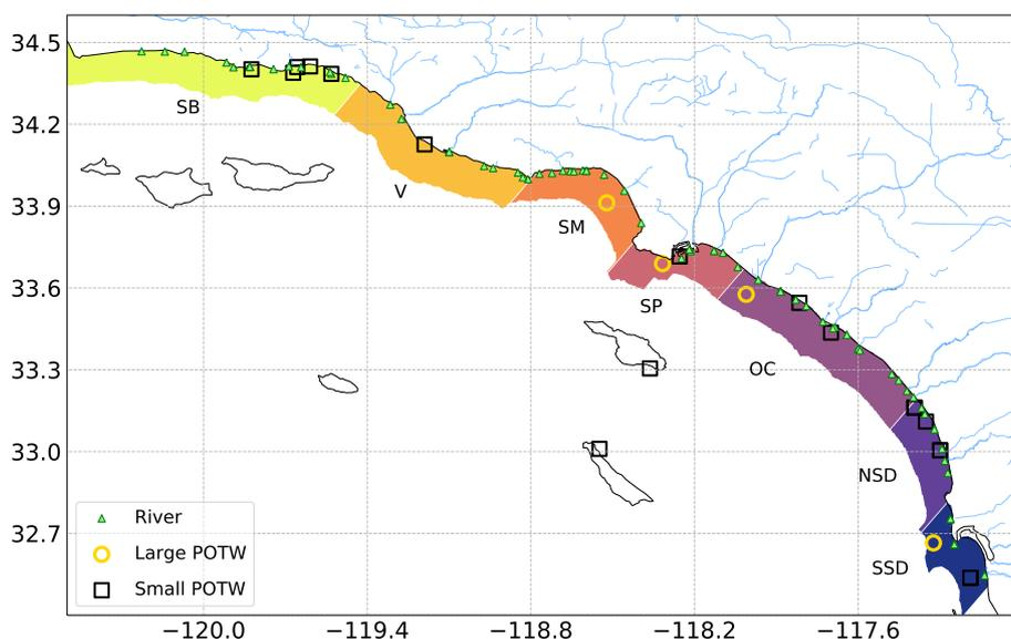
**Fig. 1.** Map of all inputs in the Southern California Bight categorized by type of input. There are four large POTWs, nineteen small POTWs, and 75 rivers. Colored sub-regions are used to summarize nutrient loading. SB = Santa Barbara, V = Ventura, SM = Santa Monica Bay, SP = San Pedro Bay, OC = Orange County, NSD = North San Diego, SSD = South San Diego.
