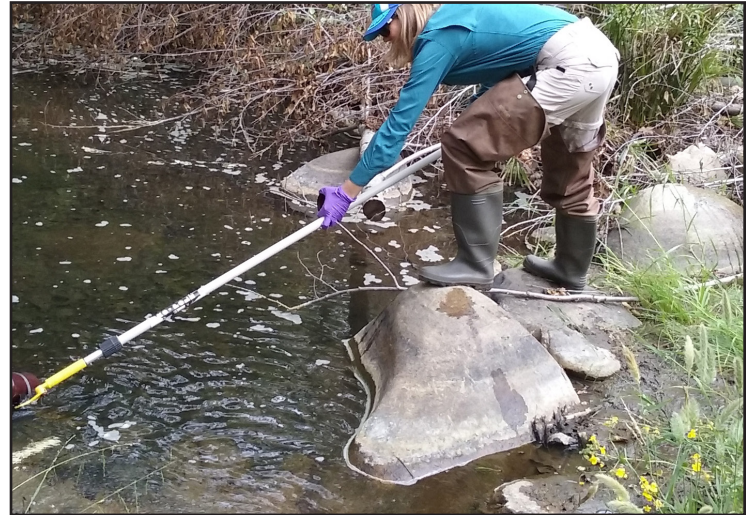
A SCCWRP field crew retrieves water samples from a stream to identify the organisms living in it via their eDNA signature.
