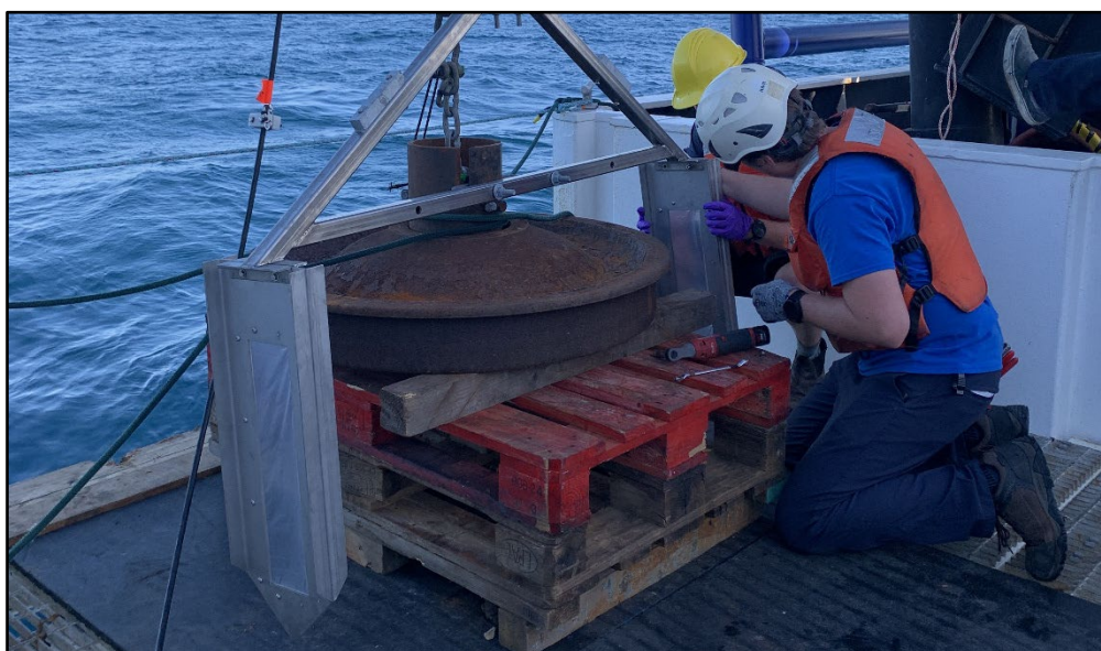
Metal spears, above, are integrated into the design of passive sampling devices to ensure the devices, upon being deployed, will stay anchored to the seafloor. Passive sampling technology, which uses a thin membrane film, was recently deployed at a former industrial waste dump site in the San Pedro Basin to measure how much of the pesticide DDT is diffusing out of seafloor sediment and re-entering the water column.
