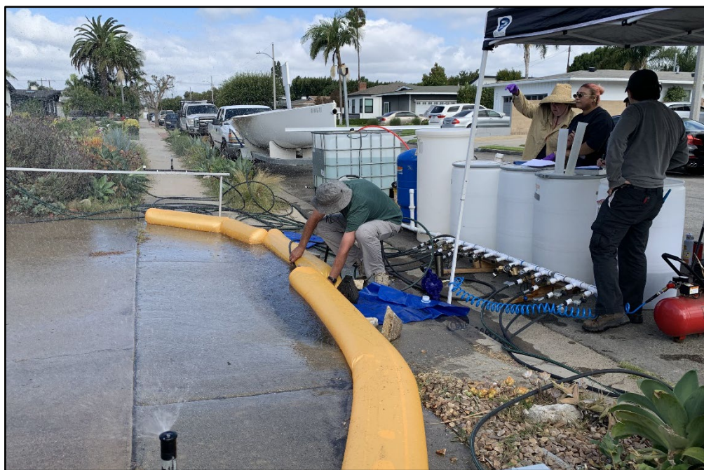
A field crew uses a custom-built rainfall generator to create controlled runoff conditions on a residential concrete driveway. The work is part of an ongoing study seeking to measure how much irrigation water and rainfall soaks into the ground vs. becomes runoff in residential areas – foundational insights that could transform Southern California's understanding of the runoff benefits associated with replacing traditional spray-irrigated turf with drip-irrigated, drought-tolerant landscaping.
