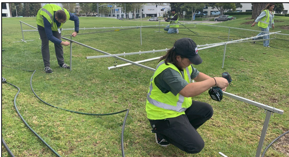
A SCCWRP field crew sets up and tests a custom-built rainfall generator in preparation for using it to measure how much rainfall soaks into the ground vs. runs off the land at sites with drip irrigation and drought-tolerant landscaping. The instrument creates controlled rainfall across a 400-square-foot footprint – more than four times as large as an earlier rainfall generator that SCCWRP developed in 2023.
