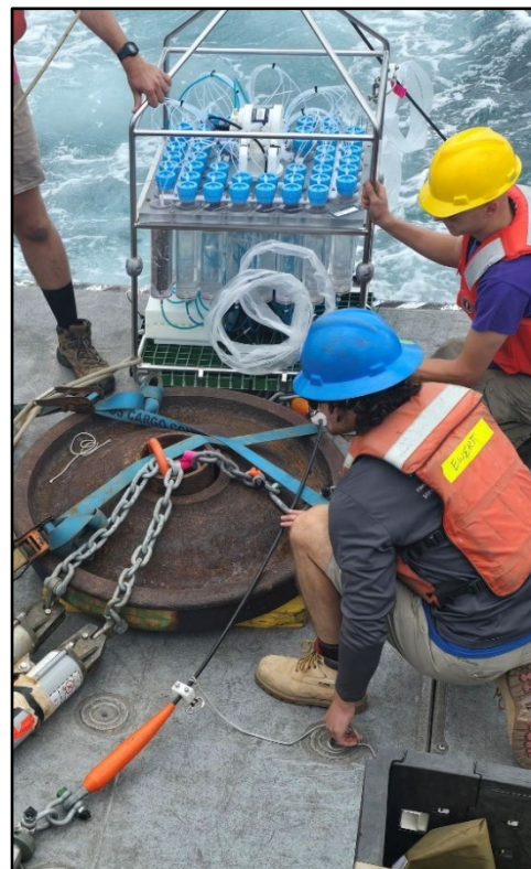
A field crew deploys passive sampling devices at an offshore site where thousands of barrels and bulk waste from production of the pesticide DDT were dumped. Researchers successfully retrieved the device after a six-month deployment.
