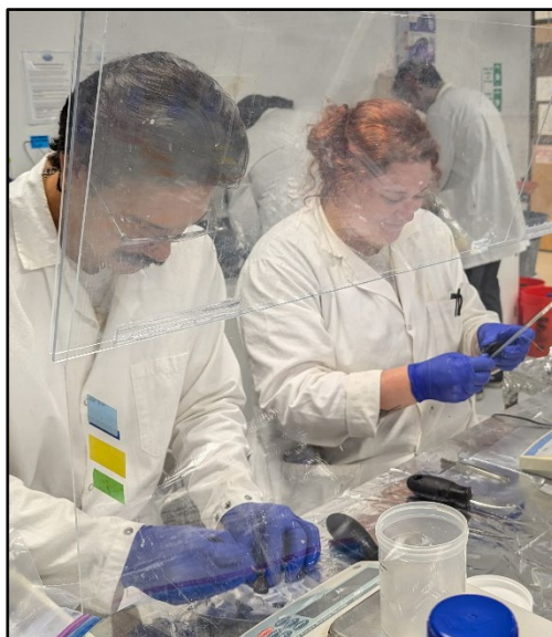
SCCWRP's Thomas Rocca, left, and Sydney Dial-Sauers dissect mussels to measure the microplastics in their tissue. The Southern California Bight 2023 Regional Monitoring Program has completed a laboratory intercalibration exercise paving the way for microplastics contamination to be measured in sediment and shellfish samples collected from across the coastal ocean.
