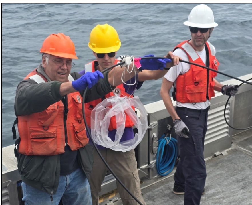
A field crew deploys passive samplers at a deep ocean dump site in the San Pedro Basin in September – part of a study that will measure levels of DDT and PCBs that are diffusing out of sediment into the water column above.
