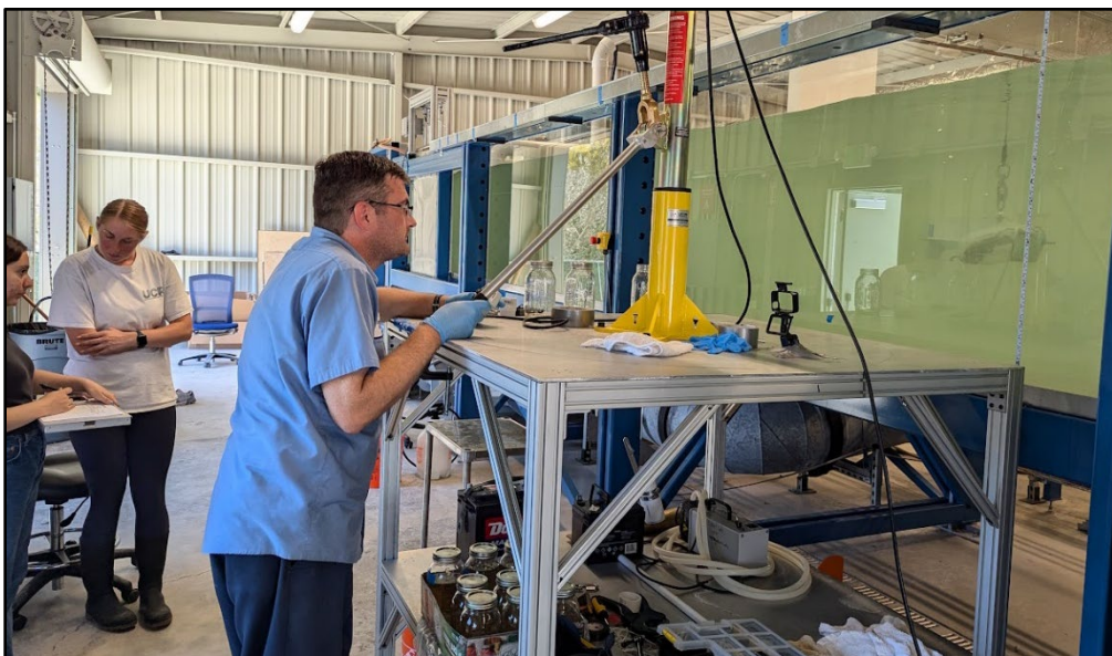
John Perna from the University of California, Riverside adjusts the flow rate of a hydraulic flume at the University of California, Santa Barbara. The flume is designed to mimic how stormwater flows in rivers, enabling researchers to test methods for sampling stormwater in preparation for measuring its microplastics content.
