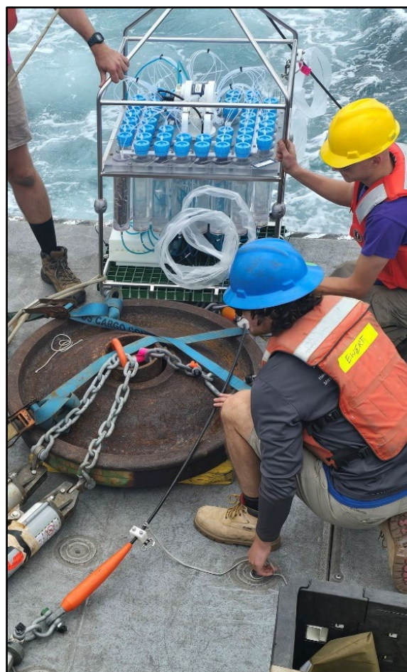
A field crew deploys passive samplers at a deep ocean dump site in the San Pedro Basin in September – part of a study that will measure levels of DDT and PCBs that are diffusing out of sediment into the water column above.
