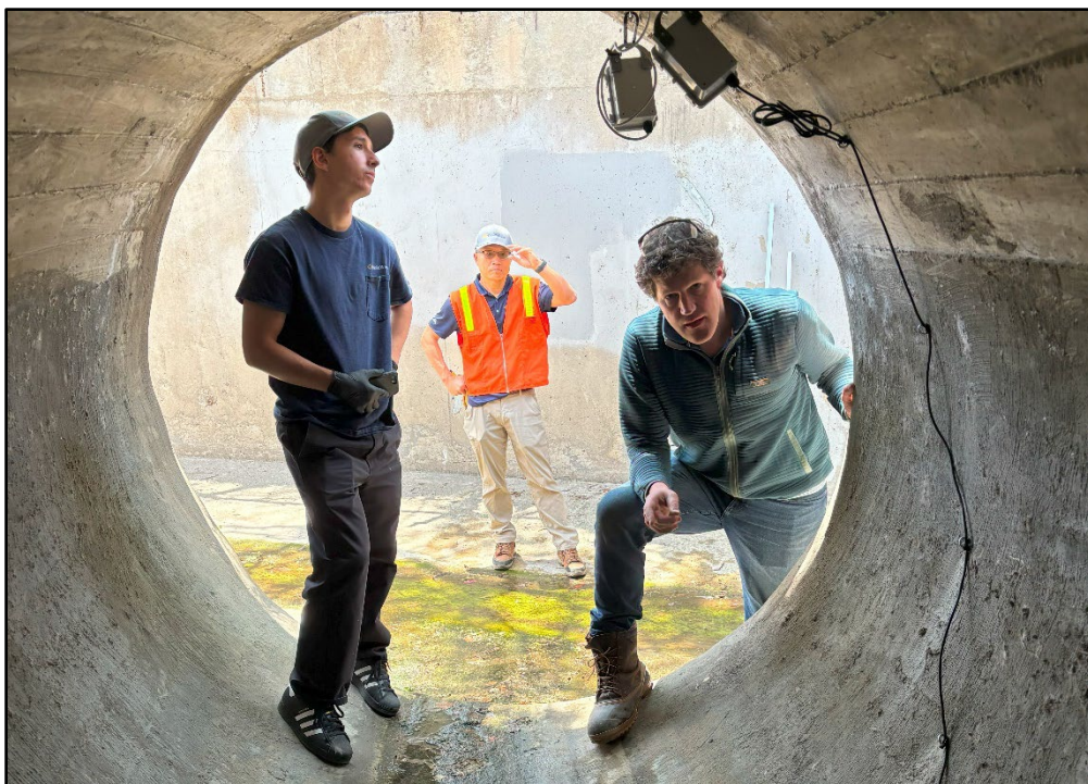
Queensland University of Technology's Dr. Dave McCarthy, right, and Orange County Public Works staff inspect low-cost field sensors installed at the end of a storm drain in Tustin. SCCWRP and its partners are investigating the feasibility and logistics of using these sensors to automate detection of illicit pollutant discharges that can pass rapidly through storm drain systems.
