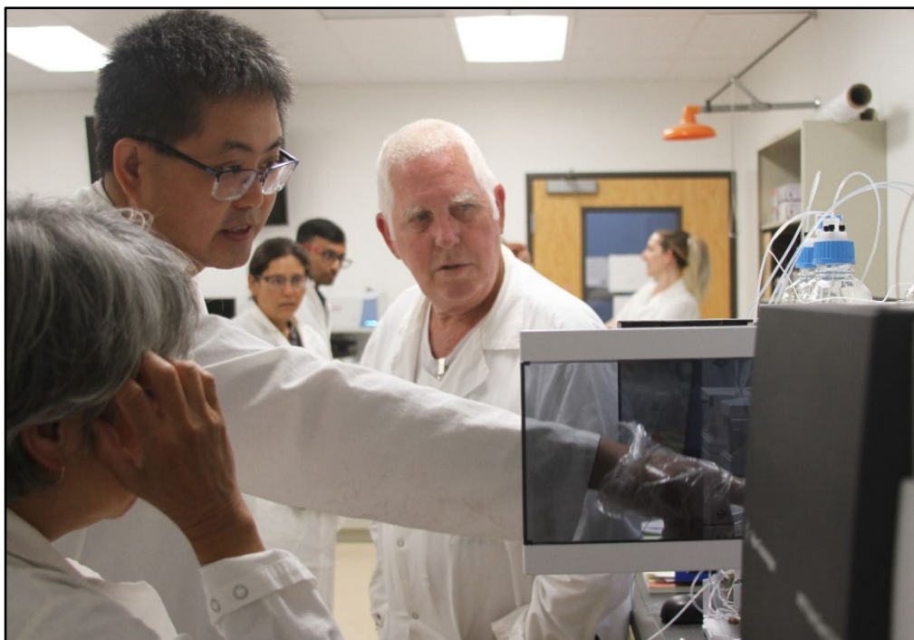
SCCWRP's Dr. Wayne Lao demonstrates how to use high-performance liquid chromatography to analyze per- and polyfluoroalkyl substance (PFAS) samples during a three-day California Environmental Laboratory Accreditation Program (ELAP) workshop at SCCWRP. The ELAP workshop was intended to teach accreditors how to measure PFAS in drinking water and environmental matrices.
