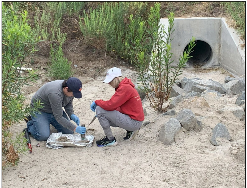
SCCWRP's Jerod Gray, left, and Liesl Tiefenthaler collect media samples from a biofiltration BMP in Orange County for microplastics analysis. Researchers are quantifying the levels and sizes of microplastic particles that have been retained inside these systems in an effort to investigate their effectiveness at removing microplastics from runoff.
