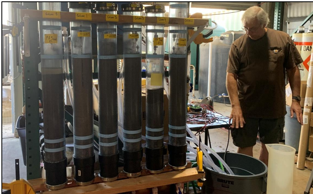
SCCWRP's Dario Diehl inspects a series of flow-through columns that have been built to mimic how runoff flows through a bioretention BMP. Researchers are working to open the “black box” for how these systems work, starting with a laboratory-scale investigation, above, that enables researchers to control and quantify a bioretention BMP's mechanistic processes.
