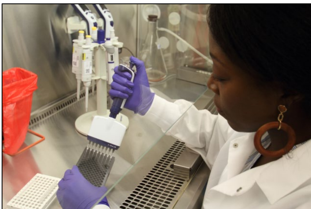
SCCWRP's Dr. Alvina Mehinto transfers cells into assay wells for a bioanalytical screening test. A newly developed set of guidance documents intended to promote international adoption of bioanalytical screening technology prominently incorporates California's recent experiences using the technology for routine recycled-water monitoring applications.
