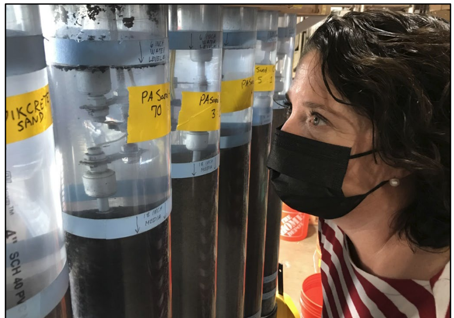
Clockwise from top left: SCCWRP's Cody Fees collects runoff as it filters through a column filled with 18 inches of engineered media; paired float switches in one of the columns monitor how quickly ponded water on top of the engineered media filters through it; SCCWRP's Dr. Elizabeth Fassman-Beck inspects water levels at the top of the columns; and runoff that has filtered through engineered media in one of the columns is collected from the bottom end to calculate flow rate.
