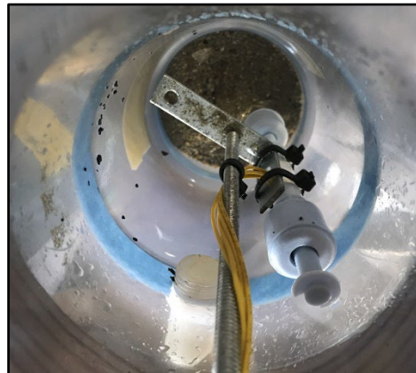
Clockwise from top left: SCCWRP's Cody Fees collects runoff as it filters through a column filled with 18 inches of engineered media; paired float switches in one of the columns monitor how quickly ponded water on top of the engineered media filters through it; SCCWRP's Dr. Elizabeth Fassman-Beck inspects water levels at the top of the columns; and runoff that has filtered through engineered media in one of the columns is collected from the bottom end to calculate flow rate.
