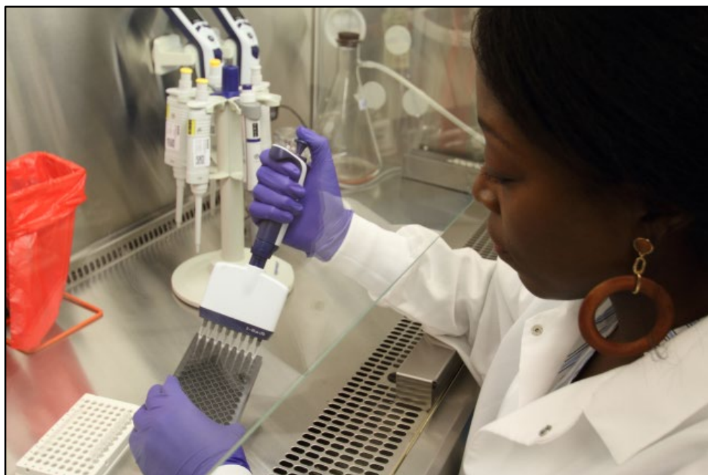
SCCWRP's Dr. Alvina Mehinto transfers cells into assay wells for a bioanalytical screening test. Researchers have demonstrated how bioanalytical screening technology can be incorporated into a regional monitoring program to help track the ecological impacts of CECs in coastal sediment.
