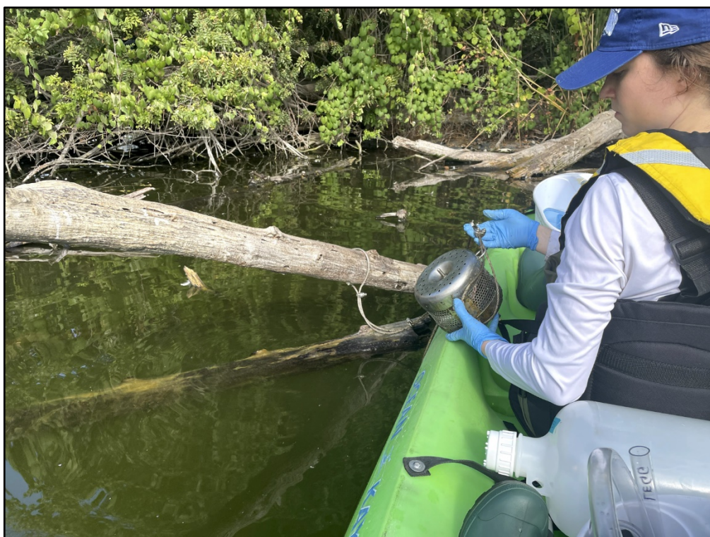
SCCWRP's Anne Holt deploys a passive sampling device in Legg Lake in Whittier Narrows Recreation Area to measure cyanotoxin concentrations in the lake, which has been tainted green by a toxin-producing cyanobacterial bloom. Researchers are examining whether existing cyanotoxin thresholds designed to protect the health of humans from cyanotoxin exposure also could be used to protect the health of aquatic life.
