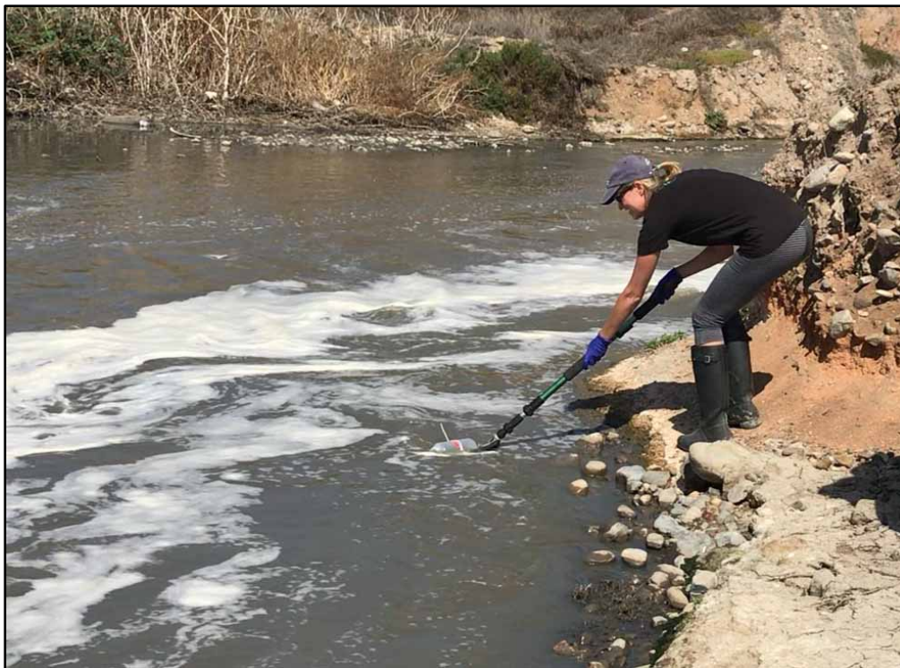
SCCWRP's Dr. Amy Zimmer-Faust collects a water sample at the site where Mexico's San Antonio de los Buenos treatment plant discharges partial primary-treated effluent into the coastal ocean. Researchers used DNA-based community fingerprinting technology to help link this sewage to fecal contamination in San Diego County during south swell events.
