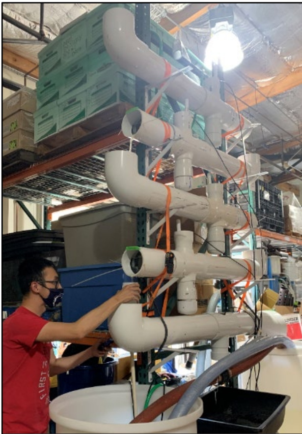
Clockwise from top left: SCCWRP's Brandon Fong calibrates flow sensors in SCCWRP's warehouse that are downstream of a series of zig-zagging pipes that create predictable rates of flow; a close-up of a weir-based flow sensor that is measuring water flowing out of SCCWRP's custom-built flow-measurement system; and an under-construction Riverside County bioretention planter receives runoff that has been redirected from a nearby rooftop to prevent discharge into storm drains.
