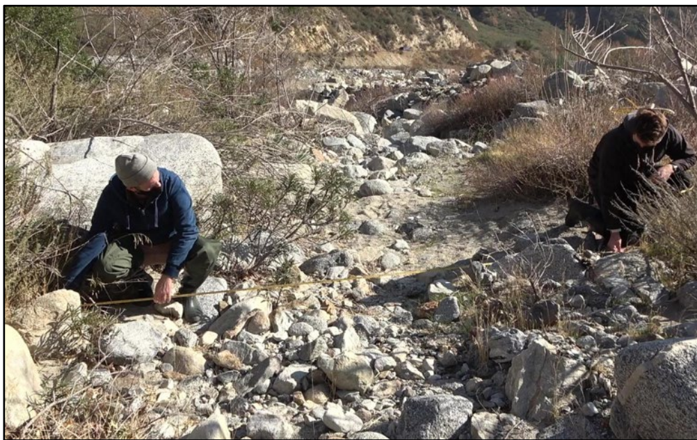
SCCWRP's Dr. Raphael Mazor, left, and Hayden Franciscus take measurements in the dry streambed of a tributary to Lytle Creek in San Bernardino County in an effort to determine whether the stream is intermittent or ephemeral. SCCWRP has developed a new tool that uses easily observable field indicators to determine the flow duration of stream reaches across the nation's arid western states.
