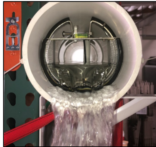
Clockwise from top left: SCCWRP's Brandon Fong calibrates flow sensors in SCCWRP's warehouse that are downstream of a series of zig-zagging pipes that create predictable rates of flow; a close-up of a weir-based flow sensor that is measuring water flowing out of SCCWRP's custom-built flow-measurement system; and an under-construction Riverside County bioretention planter receives runoff that has been redirected from a nearby rooftop to prevent discharge into storm drains.
