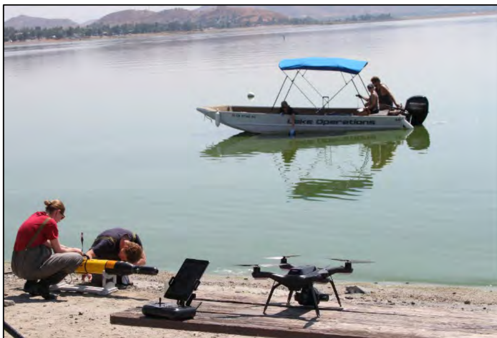
SCCWRP and its partners use an underwater autonomous vehicle, left, and a multispectral imaging sensor attached to a drone, right, to monitor cyanobacterial blooms in Lake Elsinore in Riverside County. SCCWRP and the State Water Board have developed a proposed statewide strategy for monitoring freshwater blooms that includes expanded use of remote-sensing technologies.
