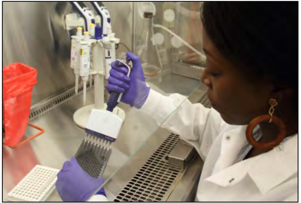
SCCWRP's Dr. Alvina Mehinto transfers small aliquots of cells into assay wells for a bioanalytical screening test. The Southern California Bight 2018 Regional Monitoring Program is screening sediment and fish tissue samples for chemical contaminants using three bioanalytical assays: the aryl hydrocarbon receptor assay, the androgen receptor assay and the estrogen receptor assay.
