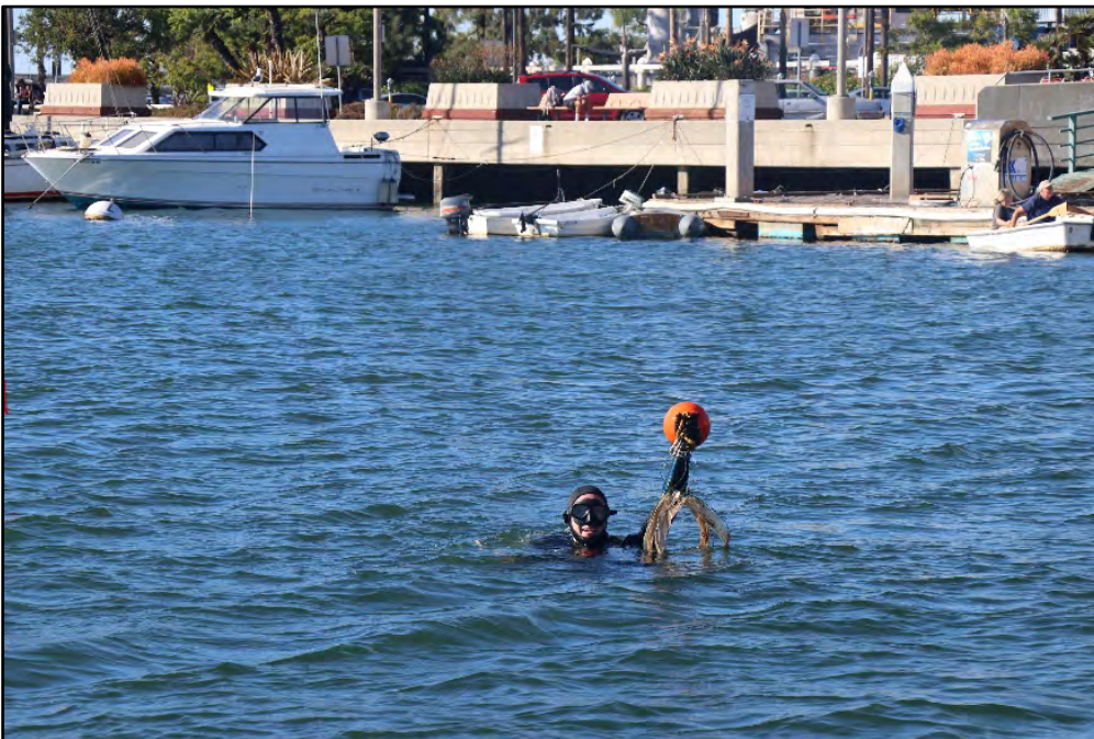
A diver retrieves a water column passive sampler from San Diego Bay. The device consists of polyethylene film that was suspended in the water for a month. Contaminants absorbed by the film will be extracted and analyzed to determine the concentration of dissolved PCBs and chlorinated pesticides.
