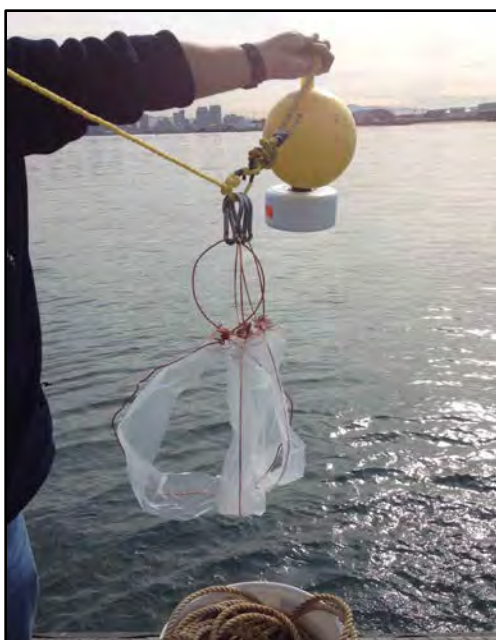
A passive sampling device consisting of rings of polyethylene sheets is deployed into San Diego Bay on a mooring. The device, which measures the concentration of legacy contaminants like PCBs and DDTs in the water column, is being used for a study examining the origins of contaminants found in San Diego Bay fish.
