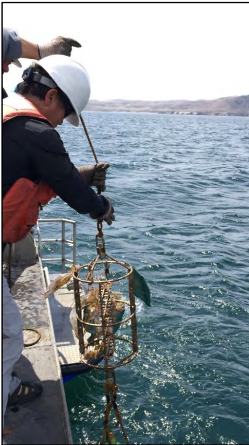
A metal cage containing passive sampling arrays is retrieved off the coast of Santa Rosa Island in the Channel Islands National Marine Sanctuary in August following a two-month deployment. The passive samplers help measure the chemical concentration of persistent organic pollutants (POPs) at the site; the findings will feed into an international study documenting background concentrations of POPs in coastal ocean water around the world.
