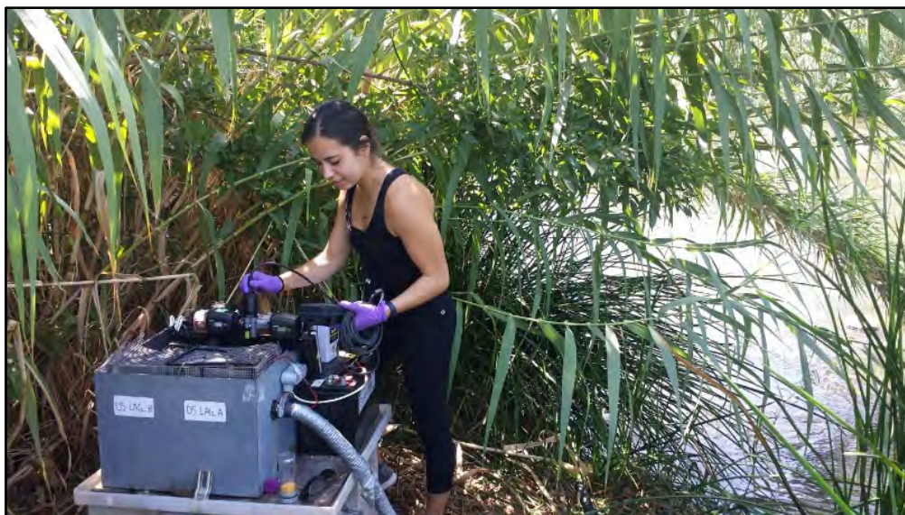
SCCWRP's Syd Kotar monitors water quality inside a mobile exposure unit on the banks of the Los Angeles River just downstream of the L.A.-Glendale Water Reclamation Plant. The units house fish that are exposed to flowing river water in real time, enabling researchers to evaluate the fish afterward for potential biological impacts from exposure to chemical contaminants in the water.
