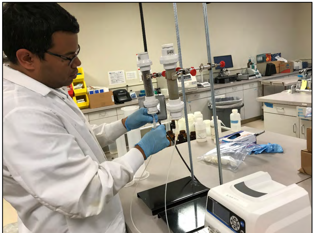
SCCWRP's Dr. Nabiul Afroz prepares to evaluate the ability of bioretention soil media to remove contaminants from stormwater runoff. The lab setup is designed to mimic much larger stormwater biofiltration units that are constructed in areas such as parking lots.
