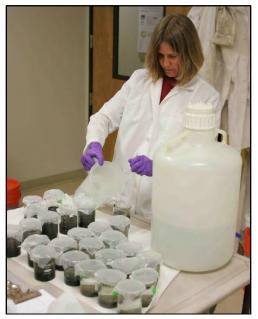
SCCWRP's Liesl Tiefenthaler prepares sediment samples collected from a site in Los Angeles Harbor for a toxicity identification evaluation (TIE) study. SCCWRP is working to optimize the design of sediment TIE studies to improve confidence in the results.
