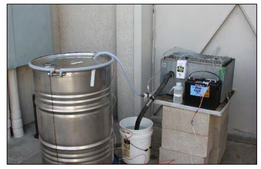
A mobile exposure unit, pictured here being tested at SCCWRP, pumps water in real time through exposure chambers that house fish. SCCWRP and its partners are setting up the units along the banks of the L.A. River for a study examining whether fathead minnow fish are impacted by CECs in the water.
