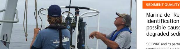
Field samplers lower a CTD (conductivity, temperature, depth) rosette into the ocean to take a variety of measurements for a synoptic analysis of ocean acidification conditions across the Southern California Bight continental shelf. The study found that Bight marine communities are being exposed to waters at or near thresholds where they can experience adverse biological effects.
