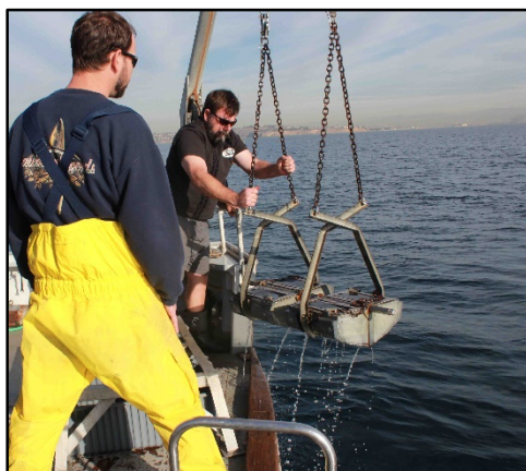
Participants of the Bight '13 program collect sediment samples to measure contamination levels. The Bight '13 Sediment Chemistry final assessment report has been published online.
