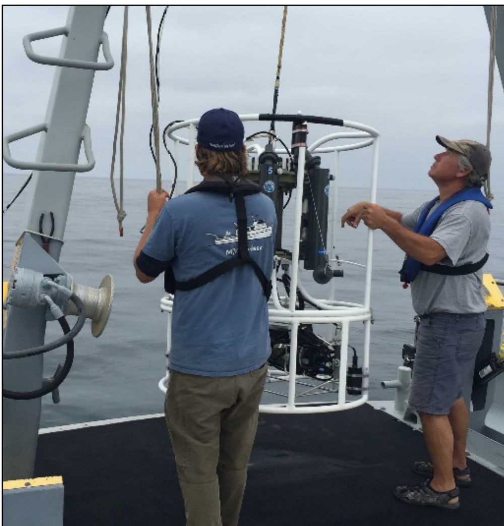
Field samplers lower a CTD (conductivity, temperature, depth) rosette into the ocean to take a variety of measurements that will help SCCWRP and its partners determine whether there are differences in dissolved oxygen levels, pH and algal blooms in different areas of the Southern California Bight as a result of discharging the nutrient nitrogen in wastewater effluent.
