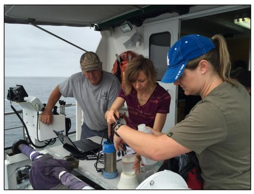
George Robertson of the Orange County Sanitation District, left, and Ashley Booth, center, and Erin Oderlin of the City of Los Angeles Sanitation calibrate and prepare an XPRIZE-developed ocean pH monitoring sensor for a test deployment in nearshore waters off Crystal Cove. All four of SCCWRP's POTW member agencies participated in the training exercise in early August.
