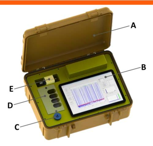
SCCWRP is planning to test the utility of a suitcase-sized droplet digital PCR instrument that could dramatically speed up how quickly beach ocean water can be tested for microbial contamination. This rendering shows the plastic housing (A), a tablet PC mounted inside (B), the sample injection port (C), the rapid-replace consumable reagent bay (D), and the target primer library (E).
