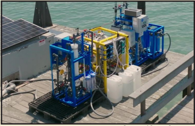
Researchers are working with Captura to investigate whether its electro-dialysis technology, pictured above on a pier in Newport Beach, has the potential to help combat global climate change as well as alleviate the effects of intensifying West Coast ocean acidification. acidification in Southern California coastal waters. Electrodialysis is one of multiple marine carbon dioxide removal (mCDR) technologies being investigated as potential solutions for the effects of climate change and coastal OAH.
