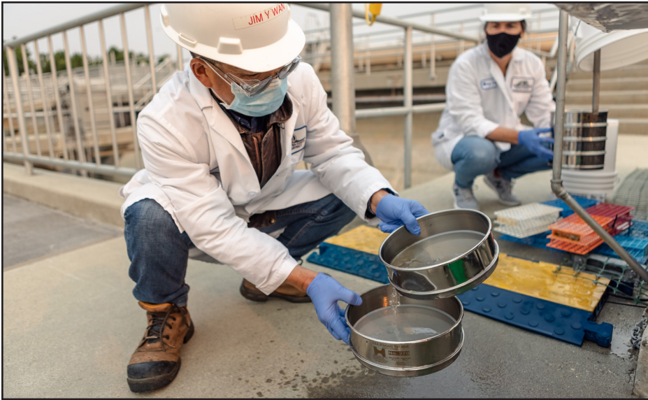
A Central Contra Costa Sanitary District team filters wastewater samples through a sieve to capture microplastic particles. The San Francisco Bay Area wastewater treatment plant is a key participant in a study measuring the degree to which wastewater discharges are contributing to microplastics loading in coastal waters statewide.
