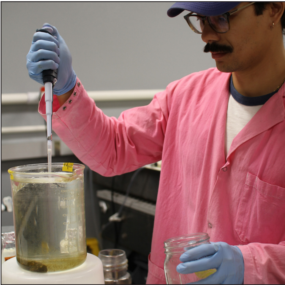
Thomas Rocca from California State University, Long Beach adds microplastic particles to a beaker containing juvenile Pacific oysters in a SCCWRP laboratory, part of a study seeking to understand adverse health effects from microplastics exposure. Among the ways that microplastics can harm aquatic life are food dilution, inflammation and oxidative stress, which can trigger cell and tissue damage.
