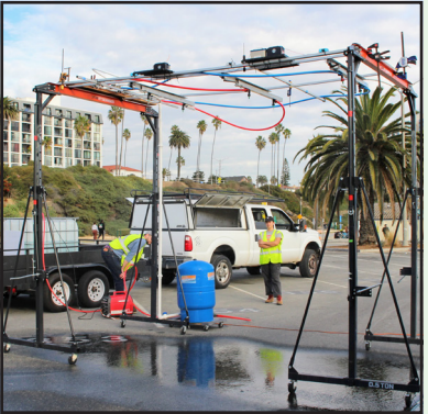
A custom-built, field-deployable rainfall generator; pictured above in a Long Beach parking lot, is being used in a study investigating the effectiveness of routine street sweeping in removing contaminants that enter storm drains and contribute to runoff pollution.
