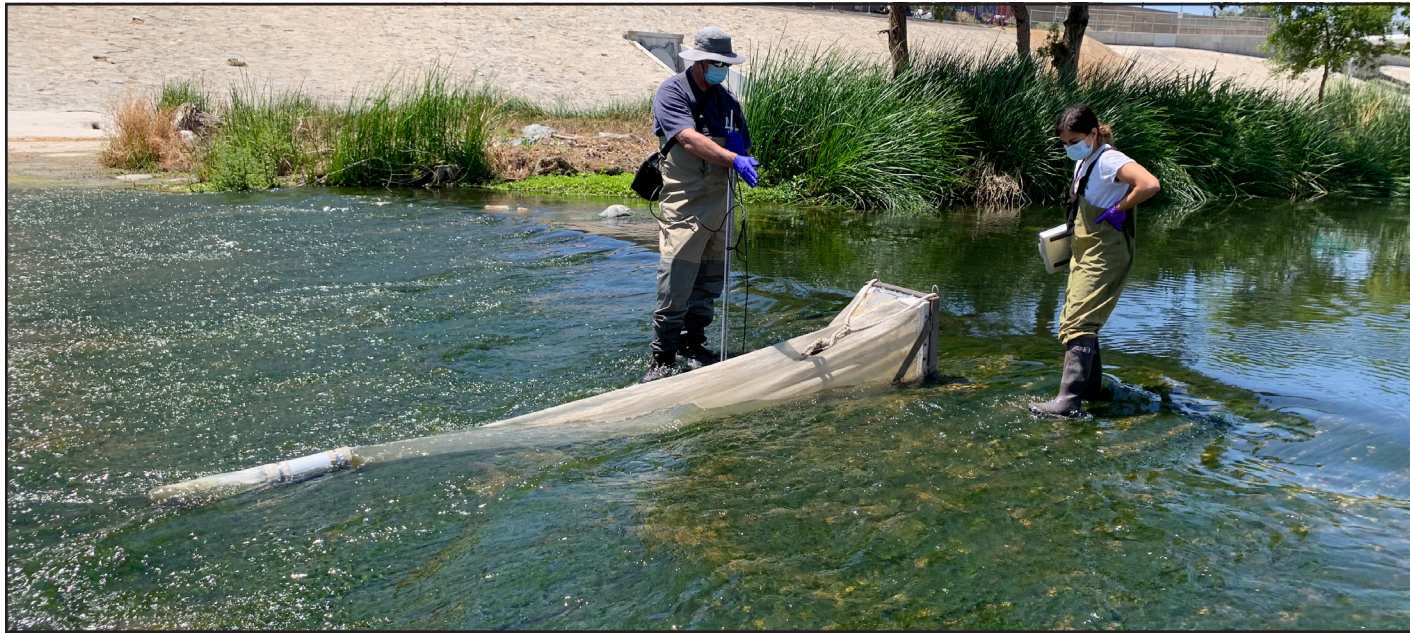
A SCCWRP field crew collects microplastics from the Los Angeles River using a mesh sampling device known as a box frame net. As water flows through the net, microplastics and other particles become trapped at the far end.
