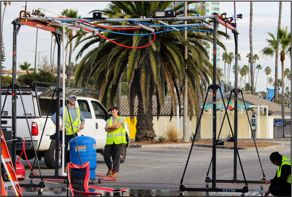
A SCCWRP field crew deploys a custom-built rainfall generator, left, to create controlled wet-weather conditions in a Long Beach parking lot. Researchers' goal is to study the effectiveness of routine street sweeping, right, in preventing a range of roadway pollutants, including microplastics, from entering storm drain systems.
