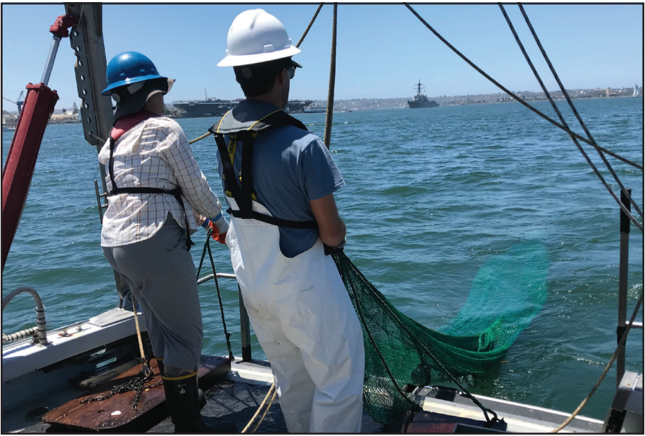
A Bight ’18 field crew retrieves a fishing trawl net that has been towed along the coastal seafloor to collect fish and other large invertebrates. The health of more than 46,000 organisms was assessed during Bight ’18 to provide an additional line of evidence about sediment quality in Southern California’s coastal ocean.
