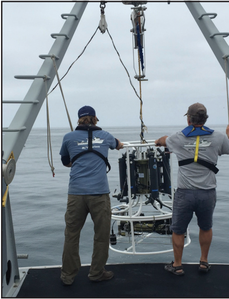
A field crew for the Bight monitoring program lowers a CTD (conductivity, temperature, depth) rosette into the coastal ocean to take a variety of measurements, including seawater pH. By tracking changing seawater chemistry, the Bight program has shown that corrosive conditions already are circulating seasonally in Southern California coastal waters.
