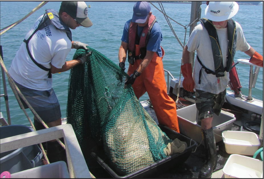
A field crew for the Southern California Bight 2018 Regional Monitoring Program retrieves a fishing trawl net that has been towed along the coastal seafloor. By collecting, counting and sorting trash from these field sampling surveys, researchers can extrapolate what portion of Southern California’s coastal seafloor contains trash.
