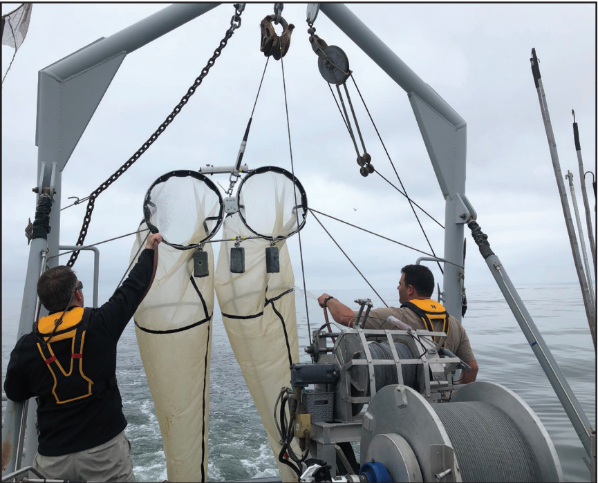
A field crew for the Southern California Bight Regional Monitoring Program uses a pair of plankton tow nets to collect small, shell-forming marine organisms vulnerable to coastal ocean acidification. SCCWRP is helping the Bight program investigate how acidification will affect coastal ecosystems – now and into the future. Page 24
