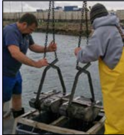
A field crew retrieves sediment samples from Los Angeles Harbor. Researchers have developed a standardized framework for assessing sediment quality to better protect the health of humans who consume locally caught seafood.
