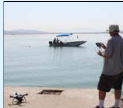
A field crew prepares to fly a multispectral imaging sensor mounted to an unmanned aerial system (UAS), bottom left, over Lake Elsinore in Riverside County. Researchers are working to adapt UAS technology to cost-effectively monitor lakes for evidence of harmful algal blooms.
