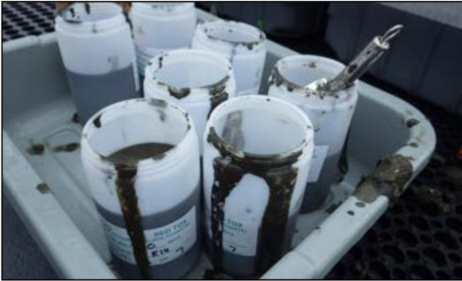
Seafloor sediment is placed in bottles in preparation for taking it to a lab for analysis. Sediment quality is evaluated using a multiple-lines-of-evidence approach to increase confidence in the findings.
