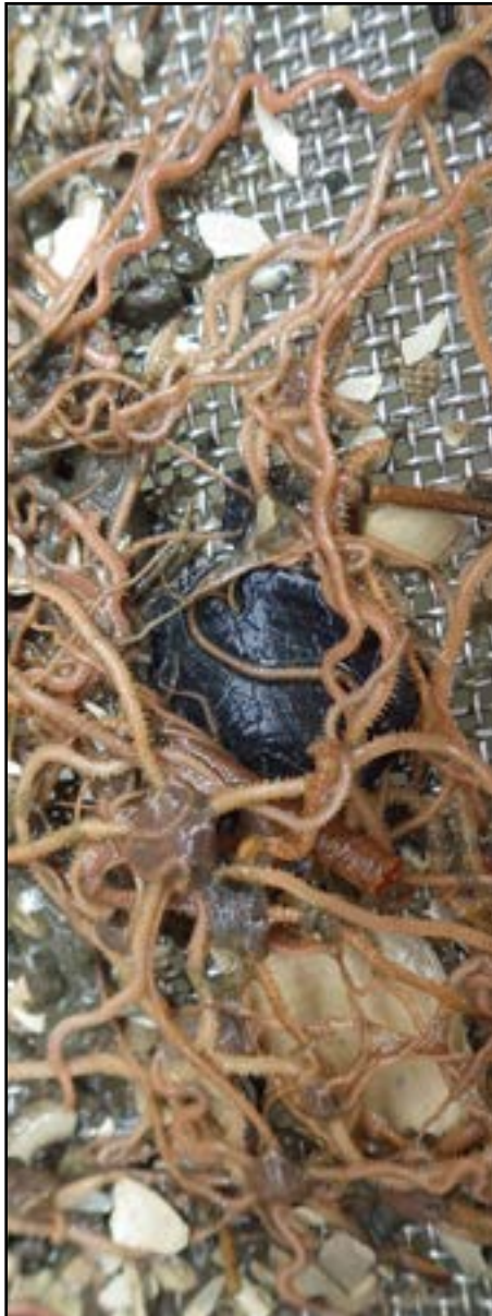
A sieve is used to isolate worms, mollusks and other organisms from sediment. The types and numbers of these organisms are analyzed to gain insights into the health of sediment-dwelling biological communities.
