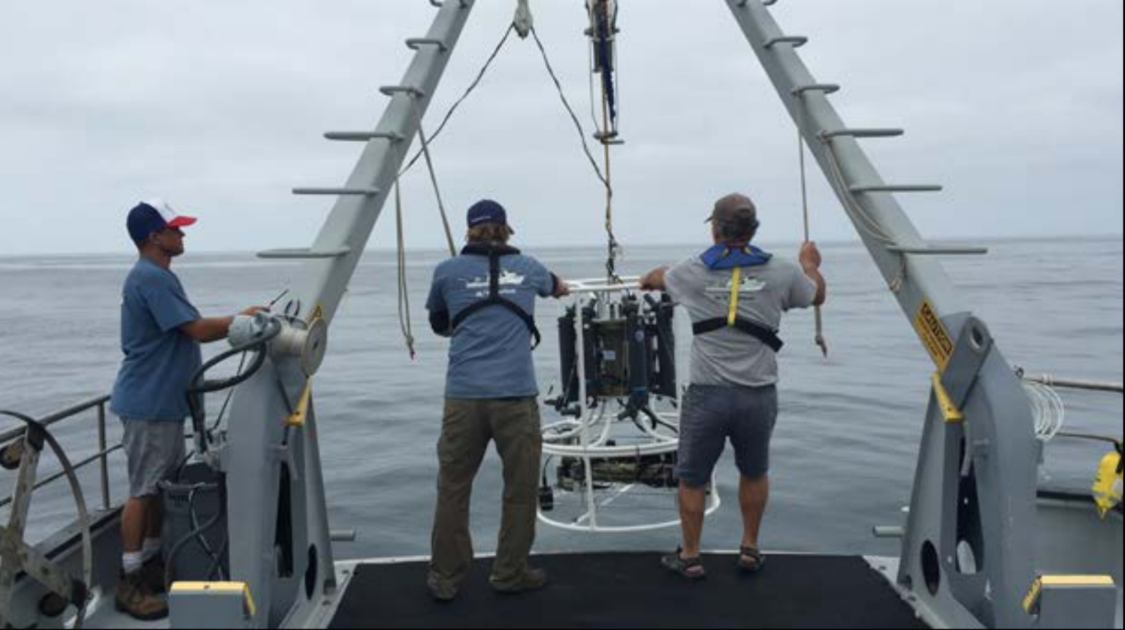
Bight '13 field samplers from the Orange County Sanitation District lower a CTD (conductivity, temperature, depth) rosette into the ocean to take a variety of measurements, including seawater pH. The study enabled researchers to get a comprehensive look at ocean acidification conditions across the Southern California Bight continental shelf.
