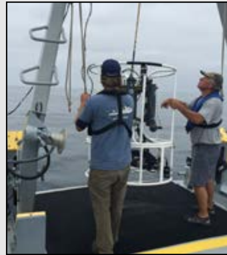
A field crew lowers a CTD (conductivity, temperature, depth) rosette into Southern California's coastal ocean to take a variety of measurements. Researchers are using this data to help validate a West Coast ocean acidification model.
