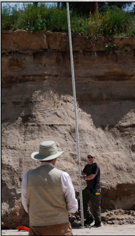
SCCWRP's Dr. Eric Stein measures the depth of Borrego Wash, an eroding creek in southern Orange County just downstream from a residential development. Over a three-year period, hydromodification-related forces lowered the creekbed by about 2 feet.
