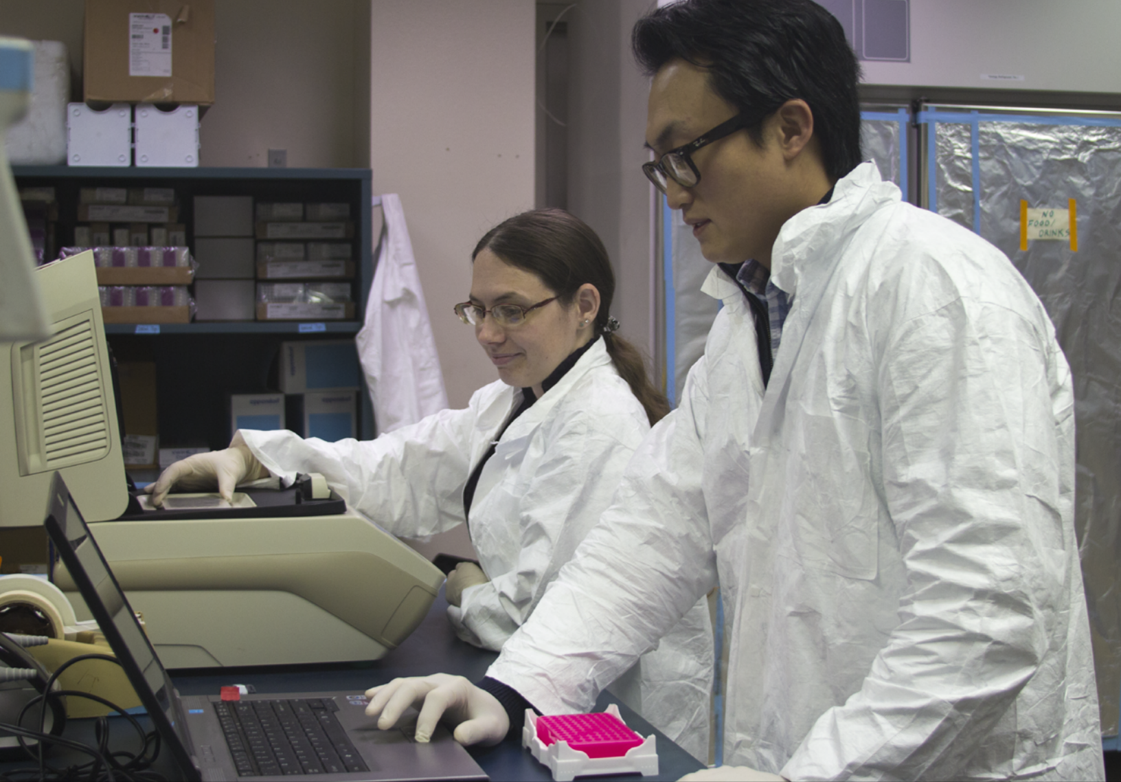
Jessica Roussos, left, and Dr. Samuel Choi of the Orange County Sanitation District's Environmental Laboratory and Ocean Monitoring Division prepare to analyze water samples for microbial contamination using their lab's quantitative PCR machine. Science conducted by SCCWRP and its collaborators has demonstrated why public-health and environmental-monitoring laboratories should invest in qPCR technology.
