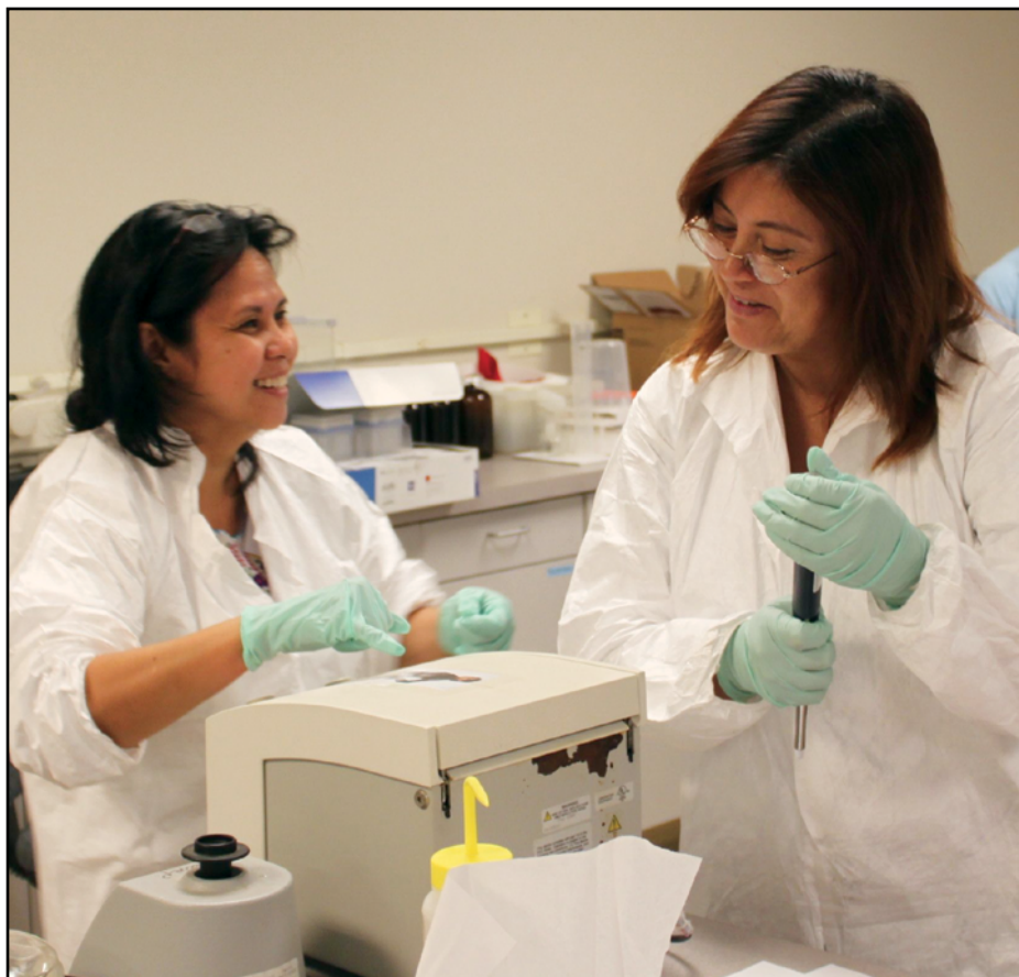
Sonji Romero, left, and Zaira Valdez from the City of San Diego's marine microbiology lab practice using a quantitative PCR machine to test water samples for microbial contamination during a SCCWRP-led training and intercalibration exercise in 2013.
